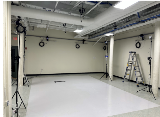
(b) Final lab design with cameras mounted, wire sleeves mounted, and wires coiled and hung against the walls
