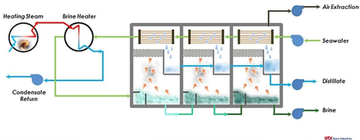
Figure 4. Multistage Flash Desalination Process, (Desalination Plant, n.d.).
