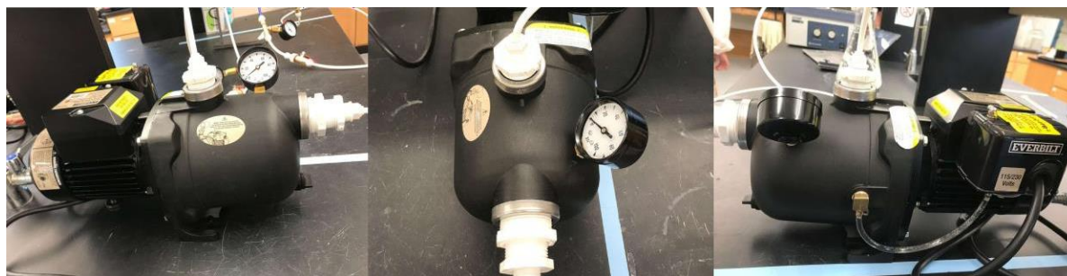
Figure 12. Everbilt ¾ HP Shallow Well Jet Pump
