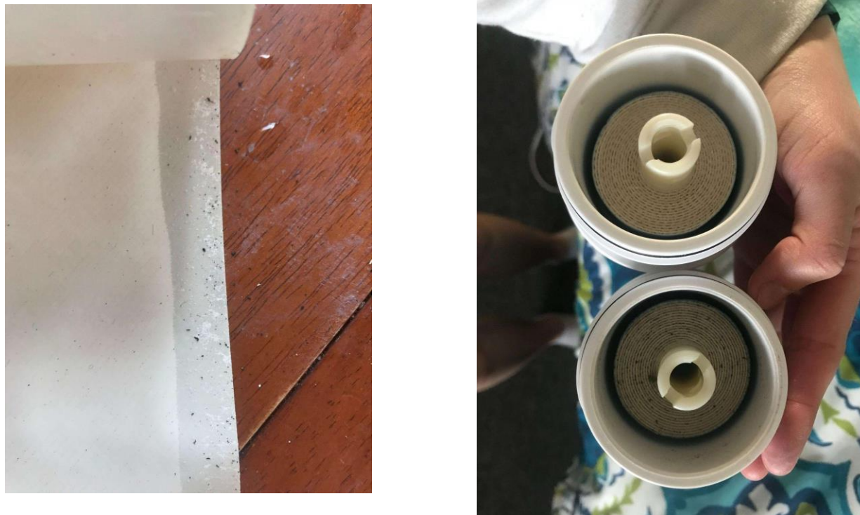
Figure 21: Visible salt on top of Salinity RO Membrane
