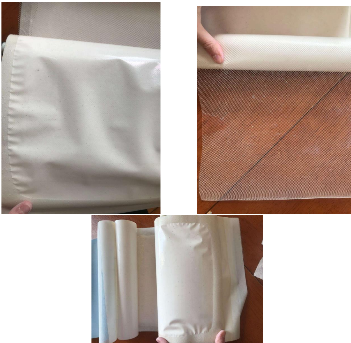
Figure 15. Layers of RO Membrane
