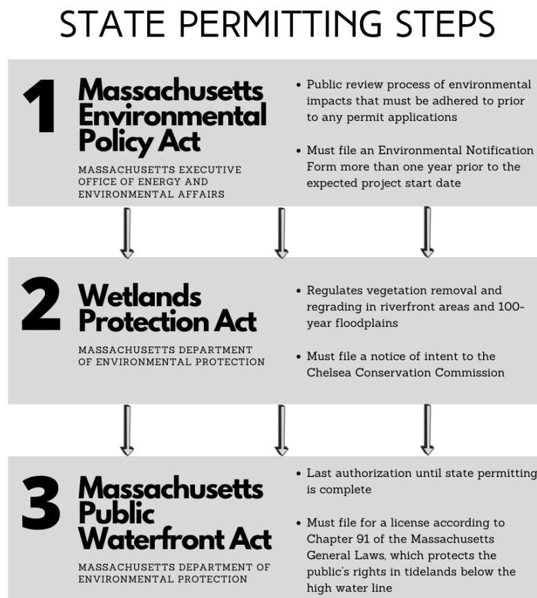
Figure 43: Major State Permitting Steps for the Proposed Project, Including the Agencies Involved. (301 CMR 11.00: MEPA regulations, n.d.; Protecting wetlands in Massachusetts, n.d., Chapter 91, the Massachusetts Public Waterfront Act, n.d.)
