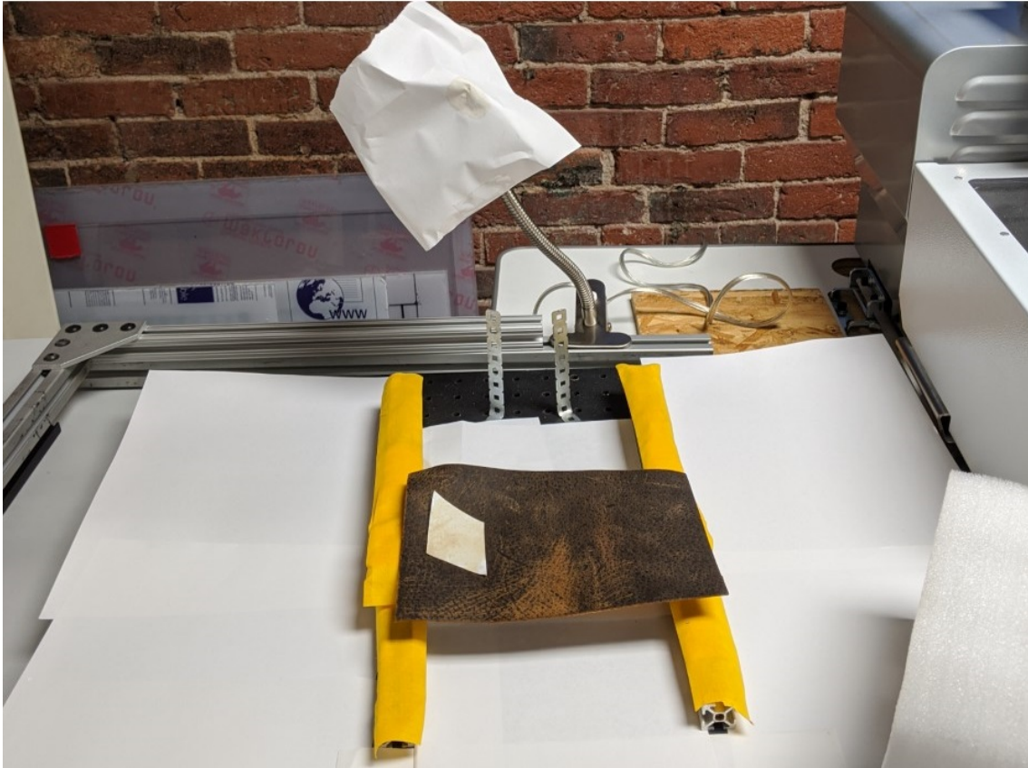
Figure 3.9: Photo of input area with fabric in the start position. The white background and yellow bars have maximum contrast with the fabric. Shaded lamp provides diffuse light for computer vision processing
