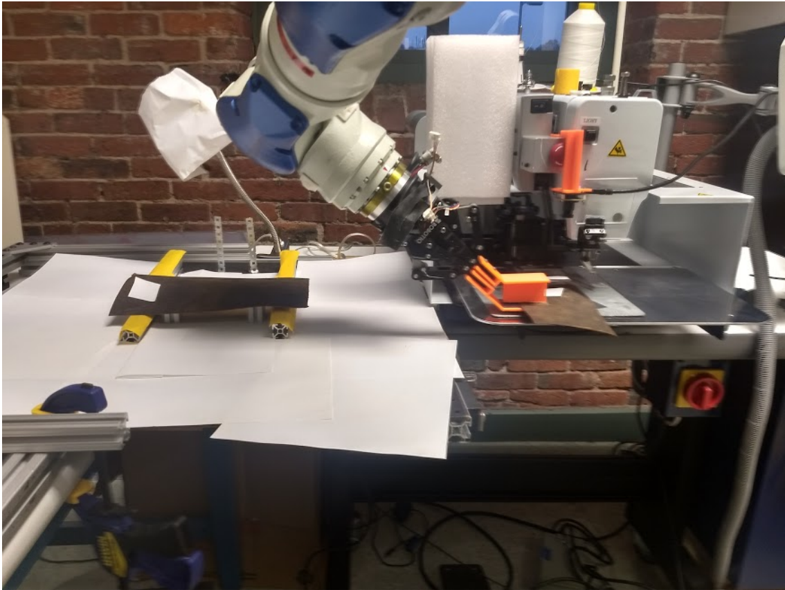
Figure 3.5: Fabric Alignment System
