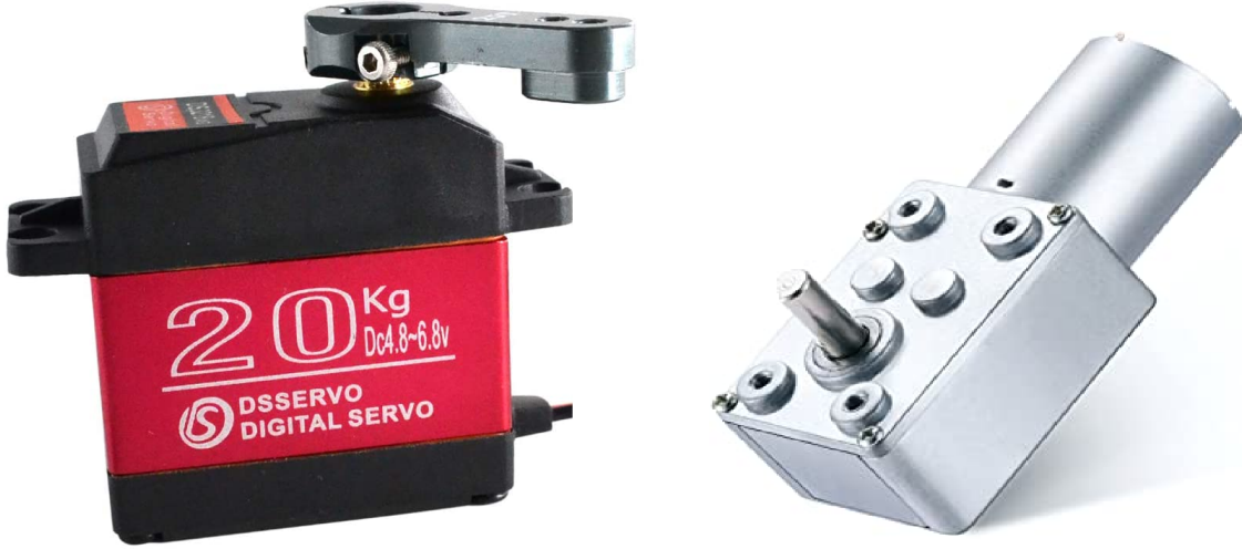
Figure 3.16: Left: Servo motor which drives the rotational joints of the Wrist, Right: Worm gear motor which drives the prismatic joint of the wrist
