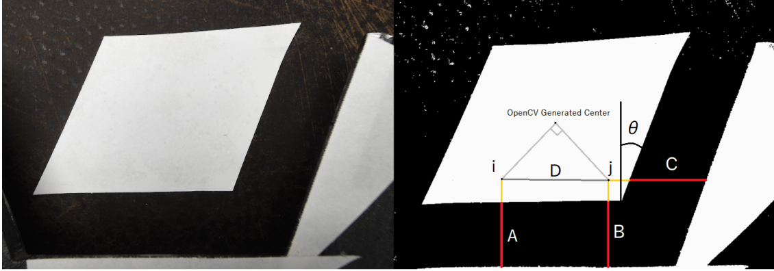
Figure 3.13: Visualization of the second stage vision processing. The generated distances A, B, and C are used along with known values D and \theta to generate the necessary alignment
