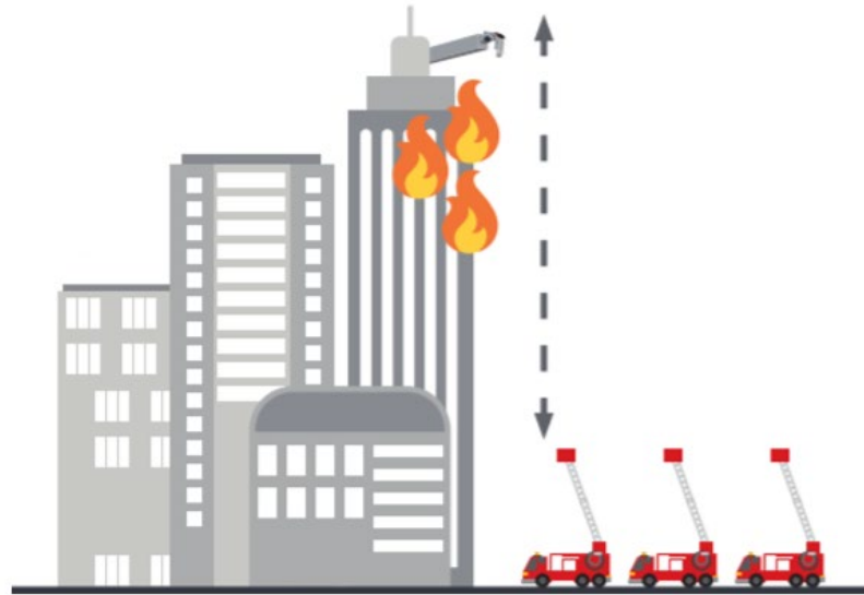
Figure 11: Spraysafe Protecting Parts of the Structure Firefighters Cannot Reach 75
