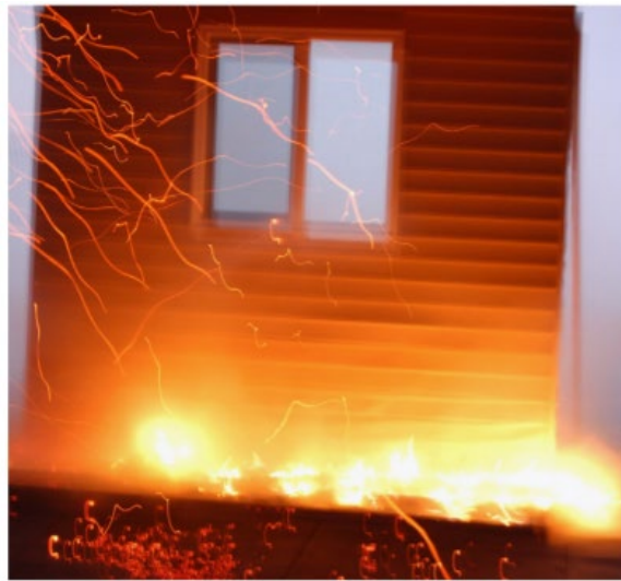
Figure 7: Flaming ignition of firebrands causing vinyl siding to melt 54
