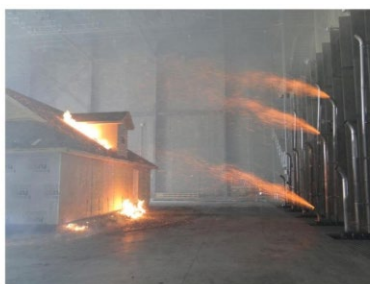
Figure 4: Burning pine needle mulch (center) and bark mulch (left). Pine needle debris next to the roof dormer also ignited 47 .
