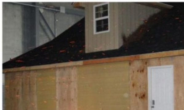
Figure 6: Firebrands accumulating near the roof dormer 51
