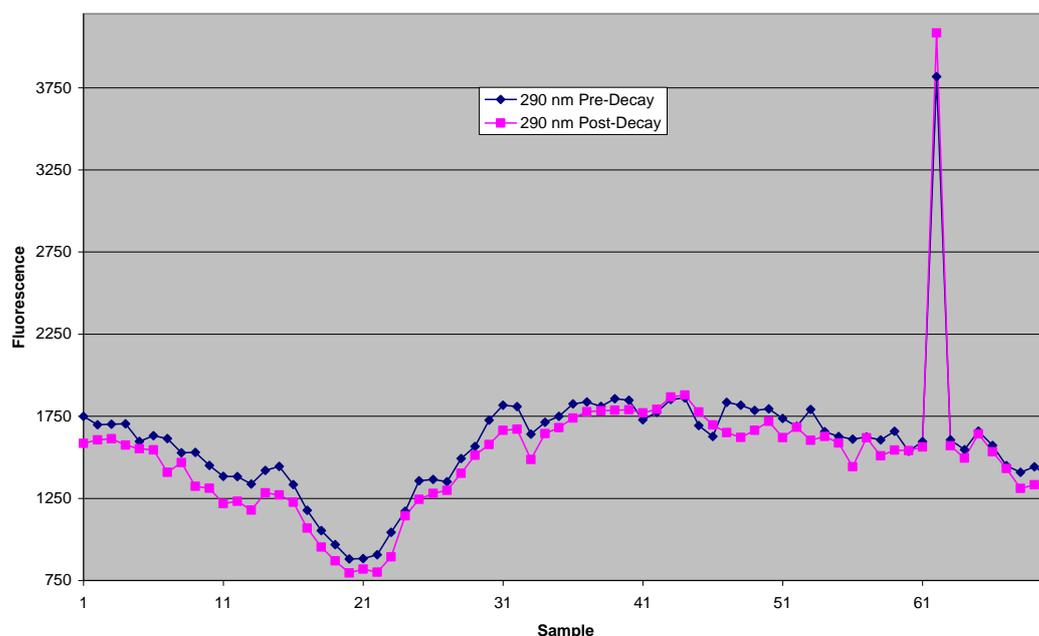
Figure 6: Fluorescence Trend versus Time at 290 nm for the Meurthe River Wastewater Treatment Plant
