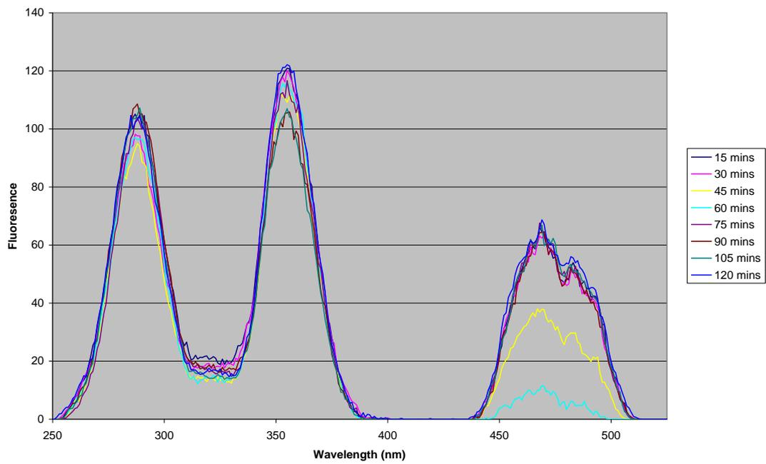
**Figure 121: DAS Optical Brightener with Tryptophan UV Irradiation Test**
