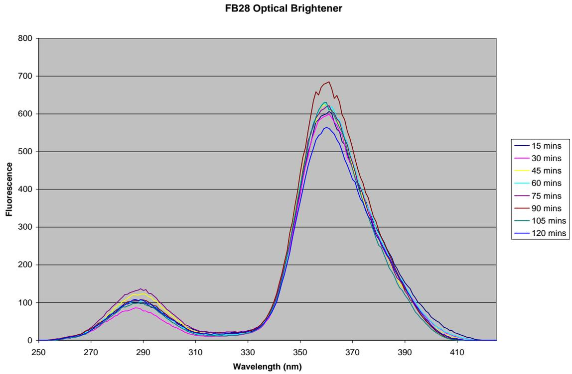
Figure 116: FB28 Optical Brightener Dilution 100 UV Irradiation Test
