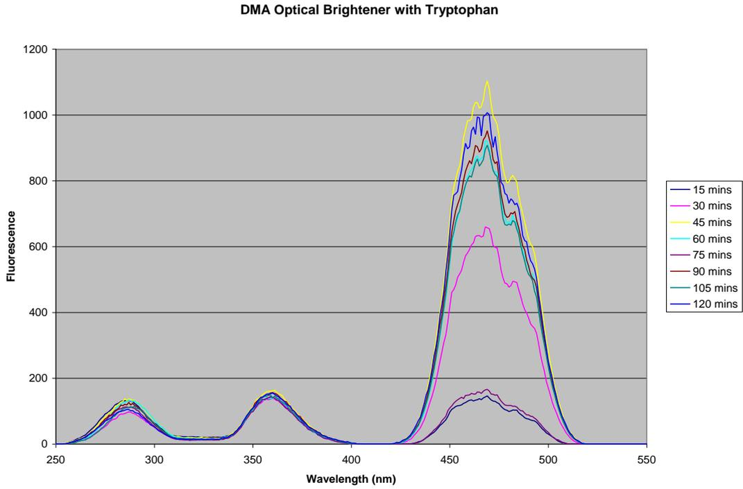
Figure 122: DMA Optical Brightener with Tryptophan UV Irradiation Test
