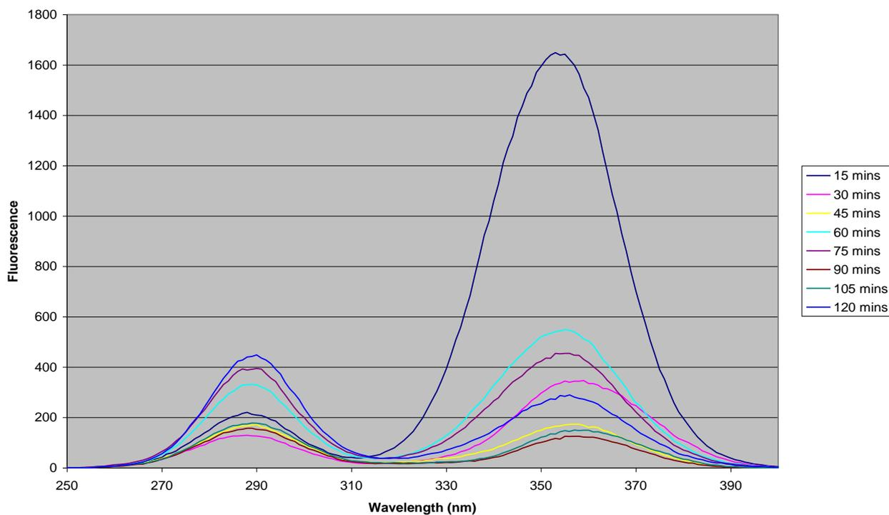
Figure 112: DAS Optical Brightener UV Irradiation
