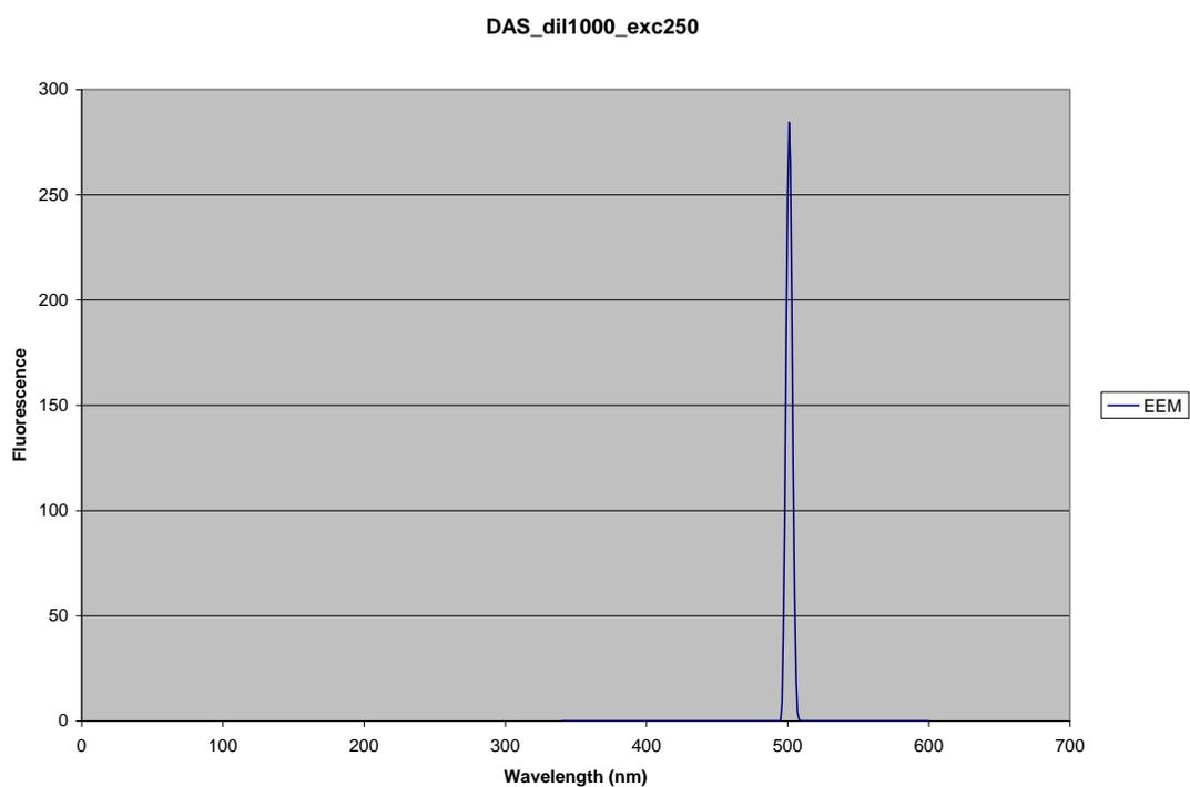
**Figure 13: Excitation Emission Matrix of DAS at 250 nm**
