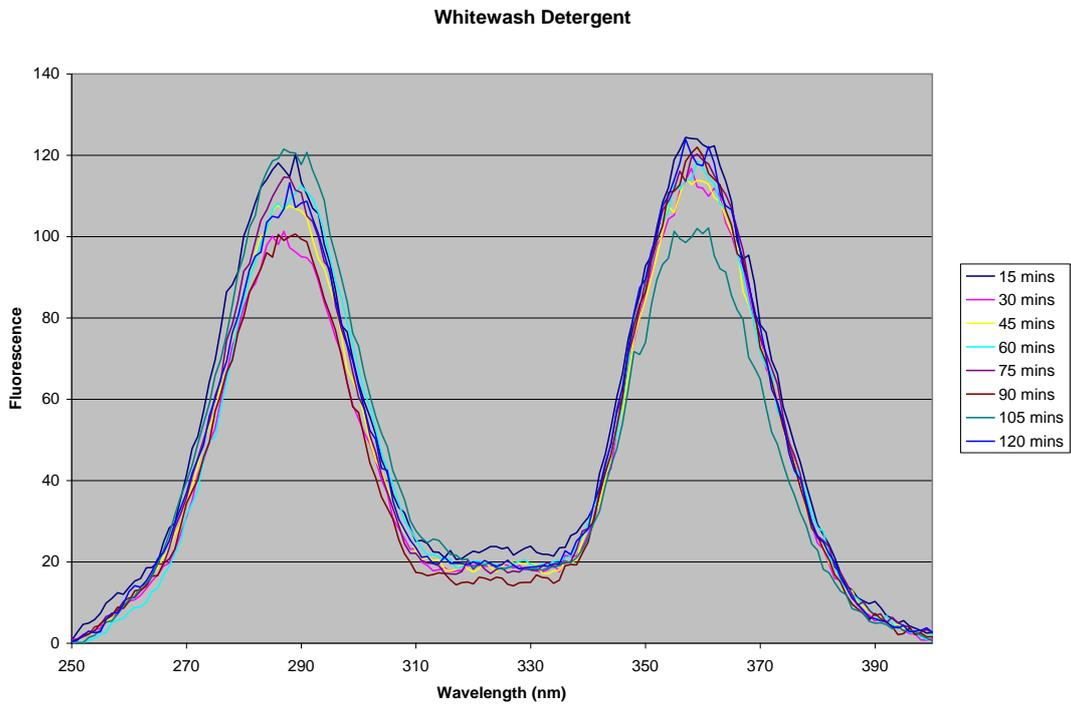
Figure 119: Whitewash Detergent Dilution 1000 UV Irradiation Test
