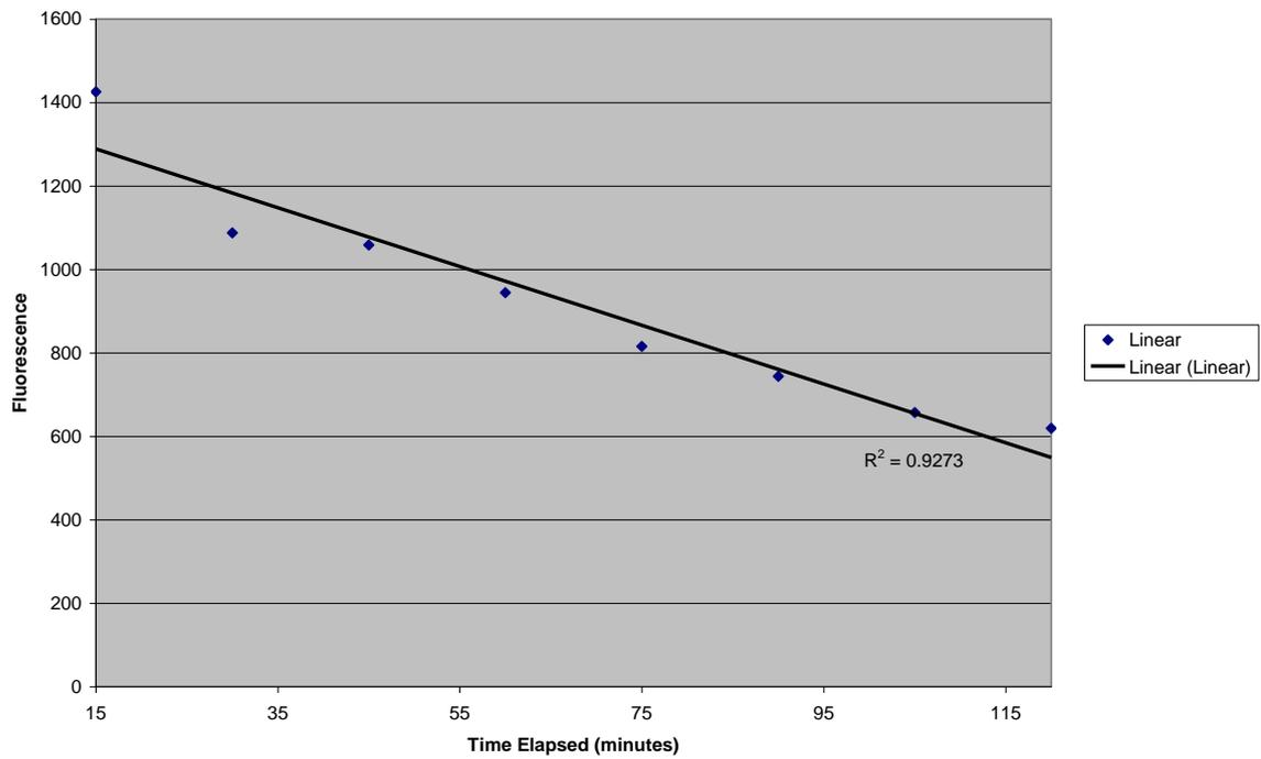
Figure 3: Linear photodegradation of CBS-X Optical Brightener
