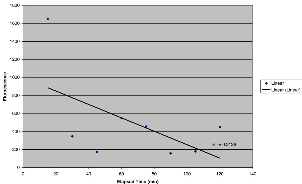
Figure 113: Linear trend of photodegradation for DAS Optical Brightener Dilution
