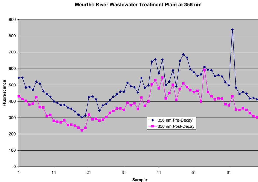
Figure 7: Fluorescence Trend versus Time at 356 nm for the Meurthe River Wastewater Treatment Plant
