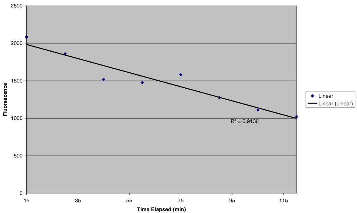
Figure 115: Linear trend of photodegradation for Ariel washing liquid
