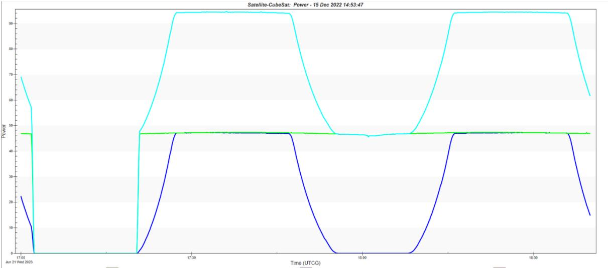
Figure 19: Solar panel power output for one orbit on June 21st, 2023
