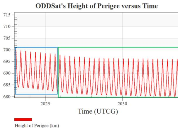
Figure 16: STK generated graph of the ODDSat's height of perigee versus time
