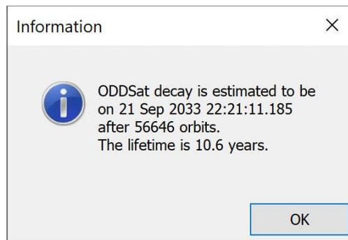
Figure 14: STK Lifetime Analysis Tool estimate for orbit-lowering from 700 to 680 km
