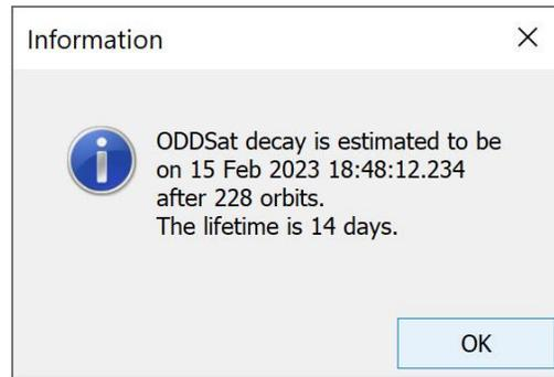
Figure 13: STK Lifetime Analysis Tool estimate for orbit lowering from 250 to 75 km
