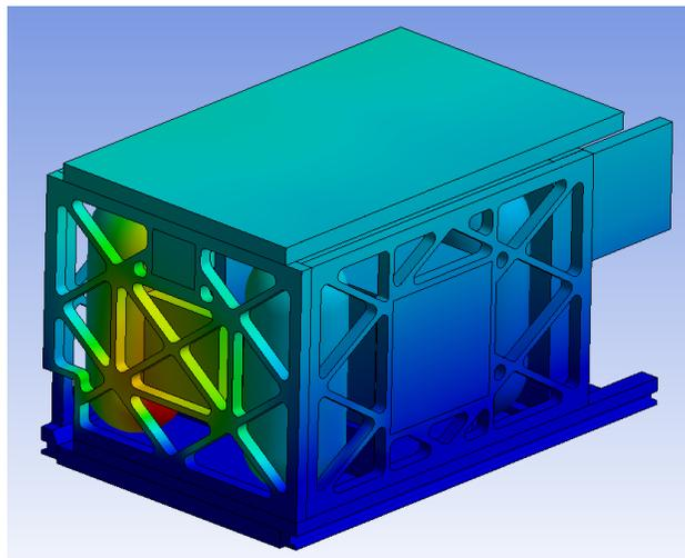
*Figure 7: ANSYS simulation results for deformation when vibration is applied on the  $Z$  axis*
