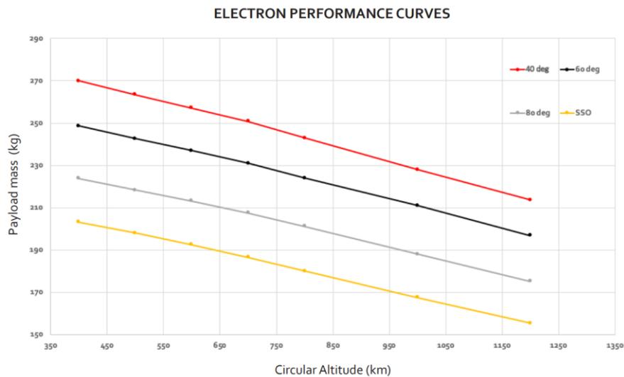
Figure 1: Electron performance curves at various inclinations [23]
