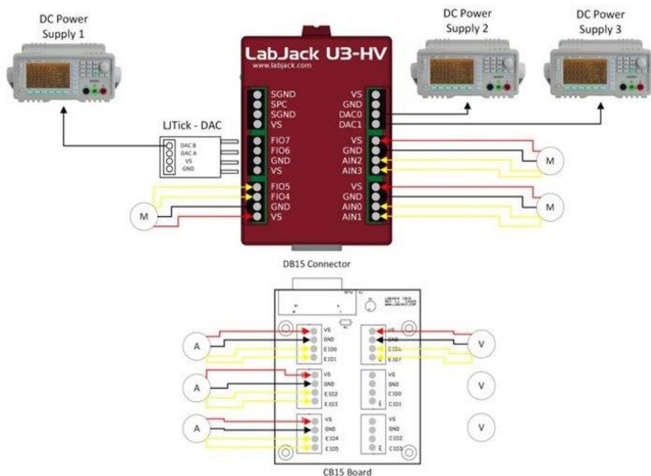
Figure 26: Wiring of LabJack, CB15 Board, and power supplies for Helmholtz cage
