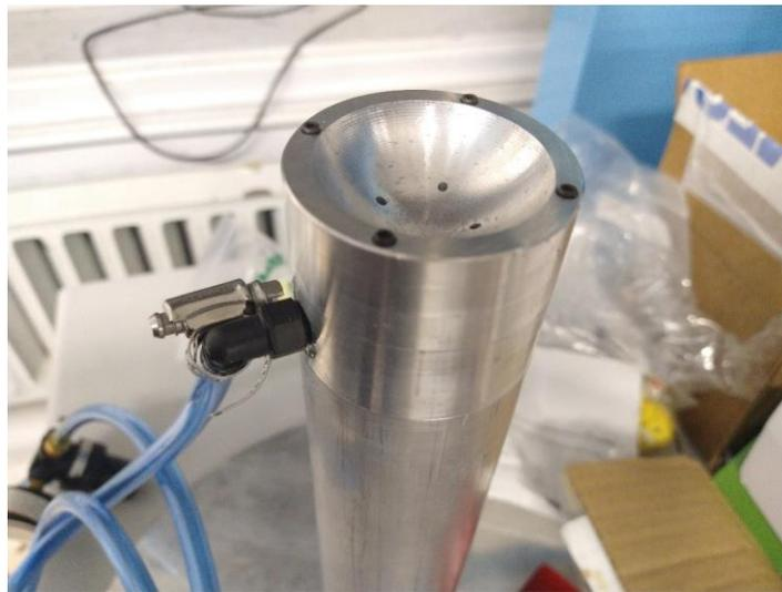
*Figure 27: The socket part of the air bearing table*
