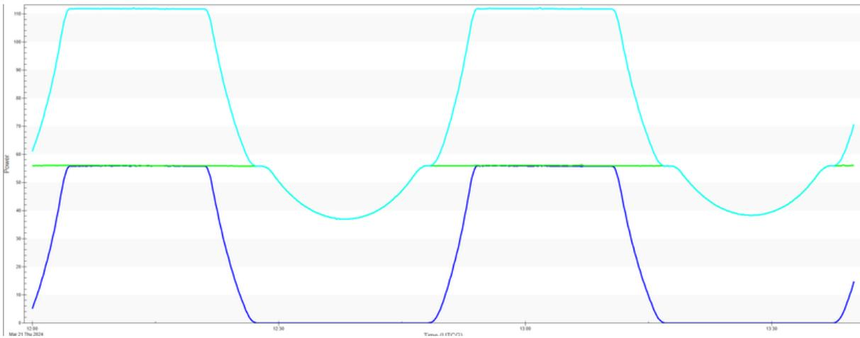
Figure 20: Solar panel power output for one orbit on March 21st, 2024
