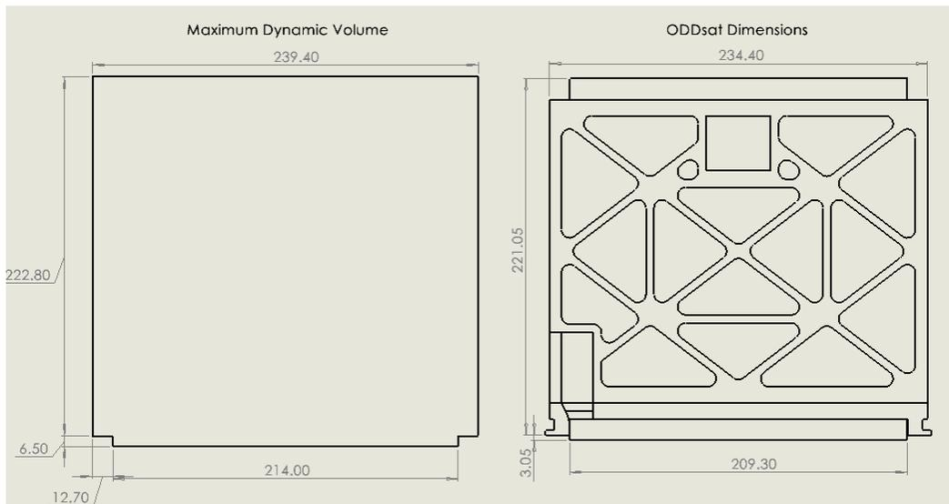
Figure 3: Comparison of the maximum dynamic volume and CubeSat dimensions.
