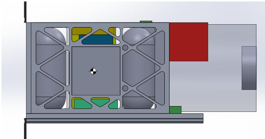
Figure 5: ODDSat in the deployed configuration, showing the center of mass.
