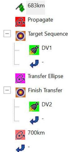
Figure 11: Hohmann transfer modeled using the Targeter
