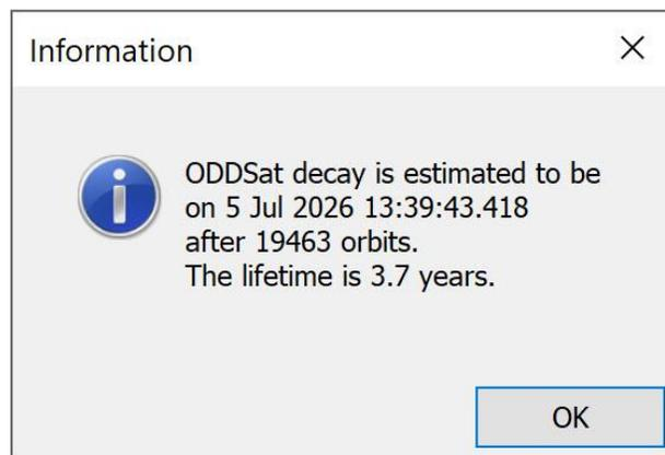
Figure 8: STK Lifetime Analysis Tool estimate for station-keeping
