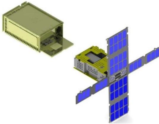
Figure 2: A 6U Canisterized Satellite Dispenser deploying a CubeSat [25]
