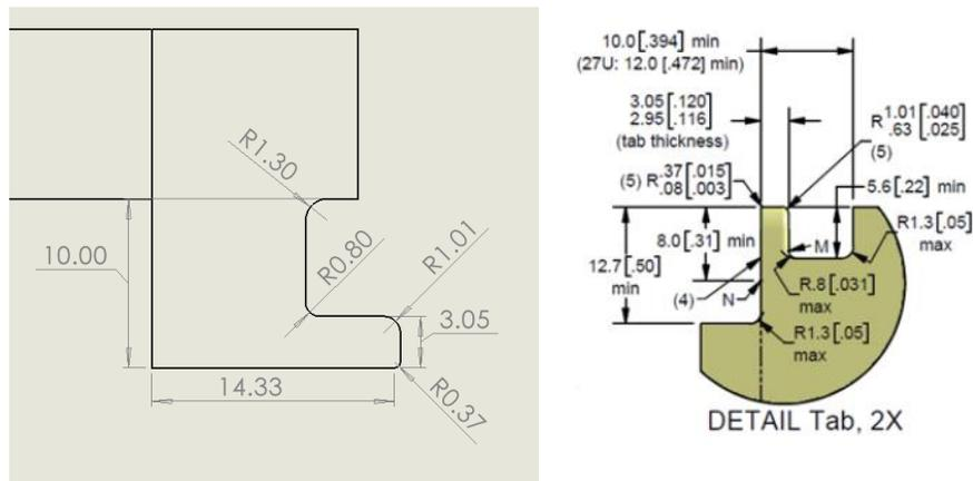
Figure 4: ODDSat's mounting tabs compared to the CSD dimensions [25].
