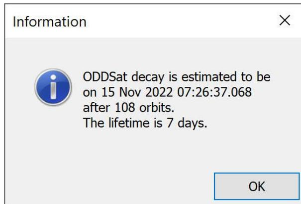
Figure 9: STK Lifetime Analysis Tool estimate for orbit-lowering from 200 to 75 km
