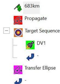
Figure 12: De-orbit burn modeled using the Targeter
