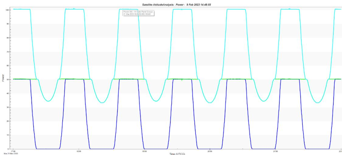
Figure 24: Solar panel power output for three orbits on March 21st, 2035
