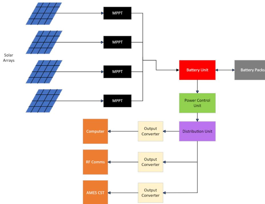
Figure 17: Schematic of general EPS internal workings and connections
