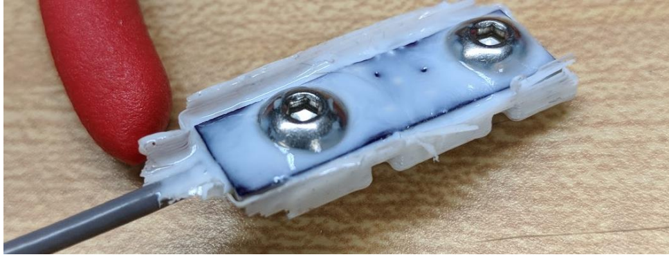
Figure 39: Untrimmed Resin Encased Electrode
