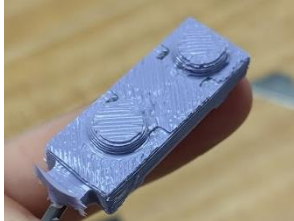
Figure 38: Covered Silicone Mold Before Trimming
