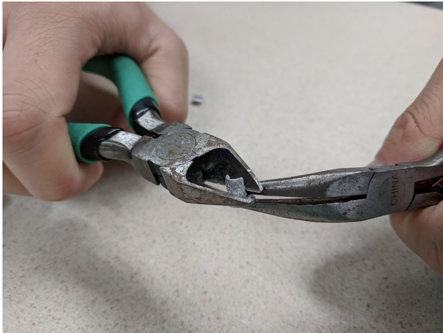
Figure 27: Using a Pair of Pliers to Help Remove the Second Flange
