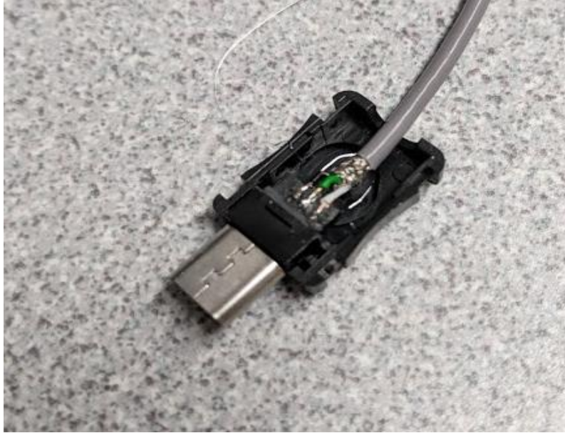
Figure 35: Micro USB B Connector Placed on Top of Hot Glue
