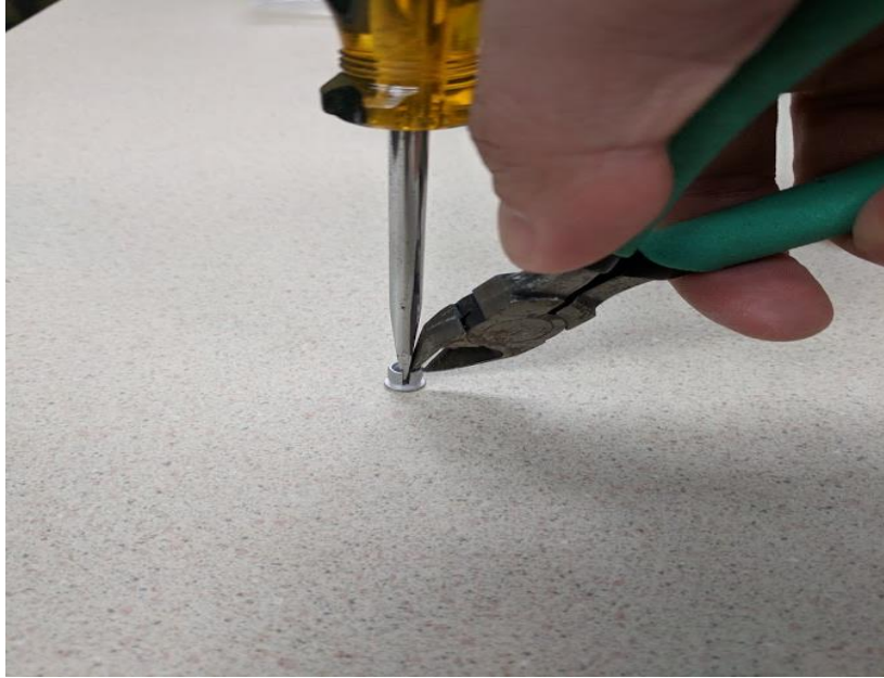
Figure 26: Using a Flat Head Screwdriver and Diagonal Cutter to Remove a Flange.
