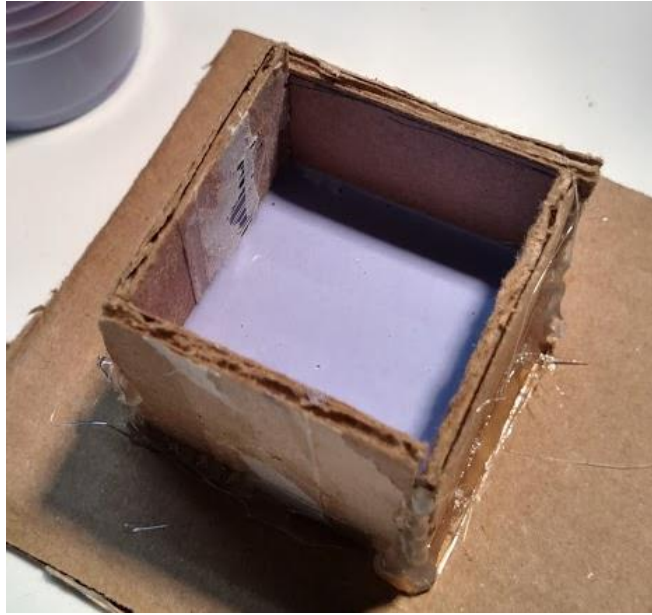
Figure 42: Poured Silicone Mold
