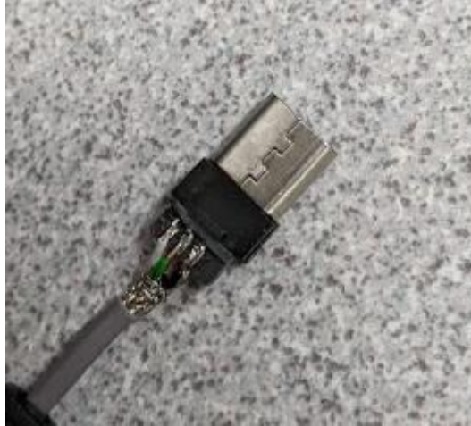
Figure 33: Top Side Wiring (White: -3.3 V, Green: SIGNAL, and Black: GND Wires)
