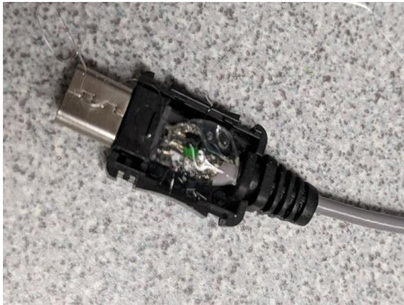
Figure 36: Hot Glue Applied on Top of the Connector Before Full Encasement
