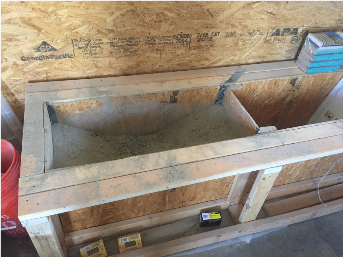
Figure 75: Robot Digging Test Rig
