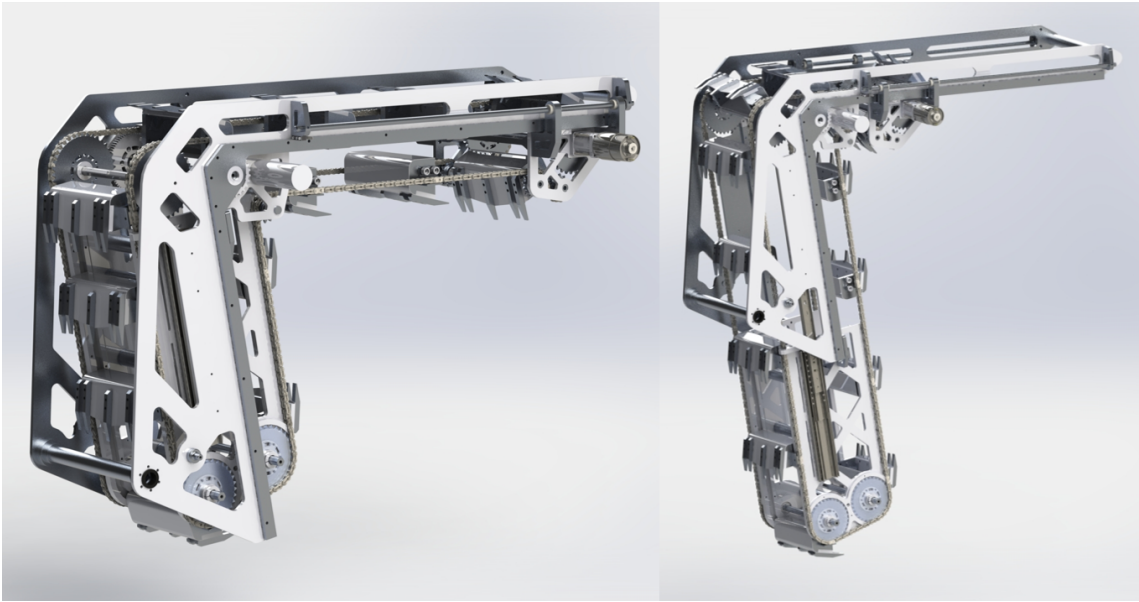
Figure 31: Collector in its retracted and extended positions
