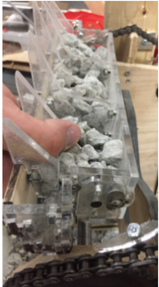
Figure 27: Rocks collected with improved teeth
