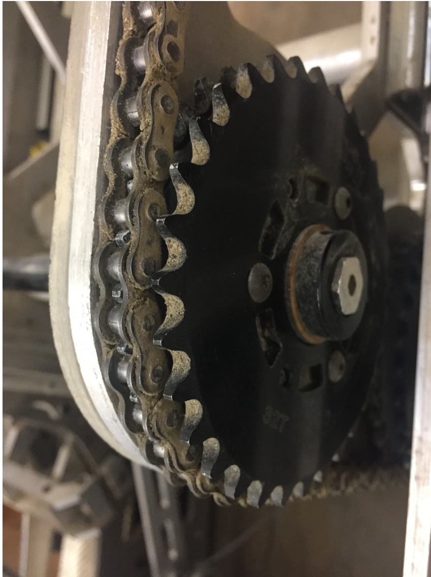
Figure 63: Outer Sprocket to prevent chain slip
