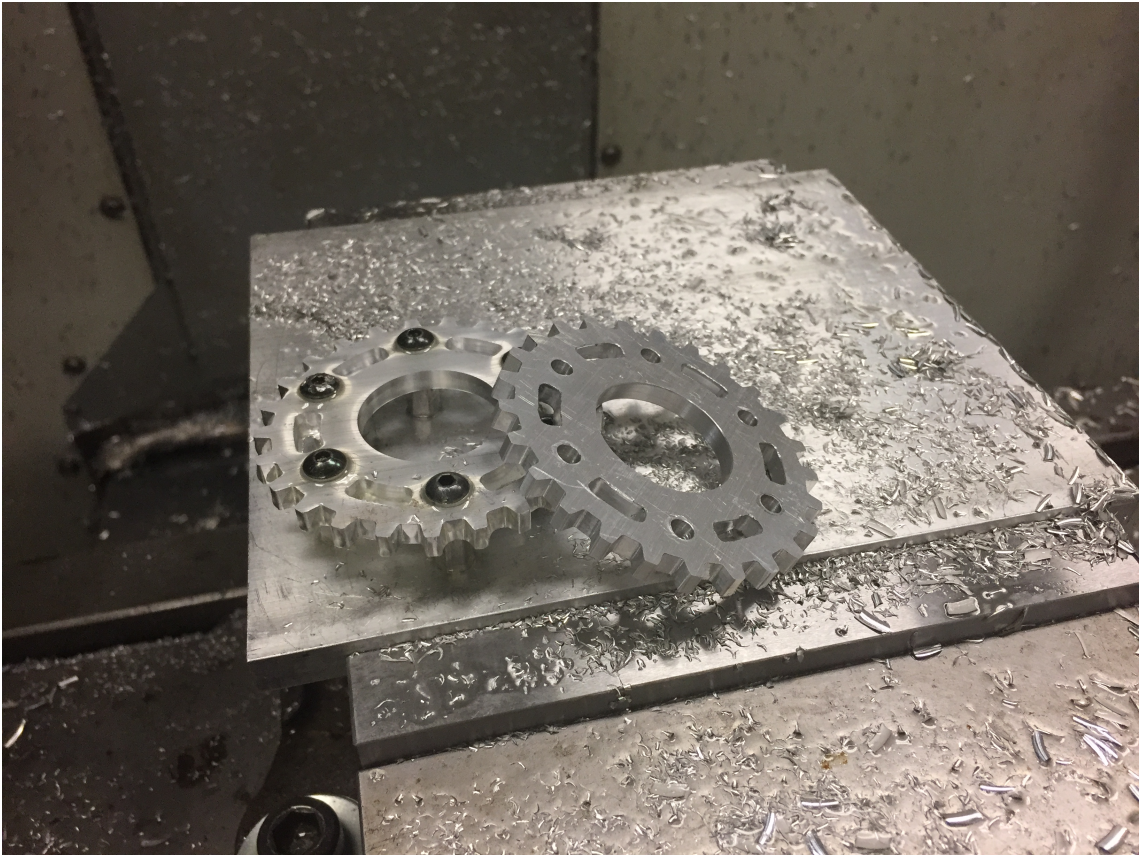
Figure 80: Sprockets for Regulator Tape
