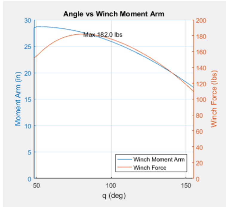
Figure 45: Winch Force Curve
