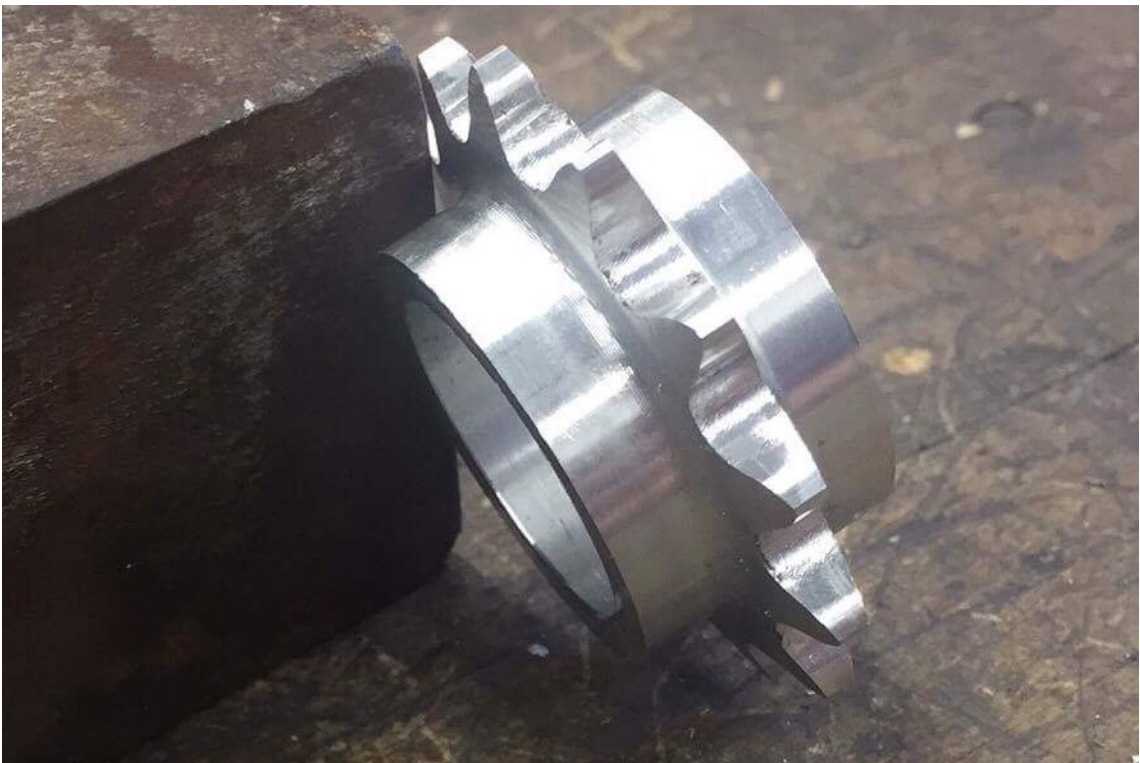
Figure 81: Custom Idler Sprockets
