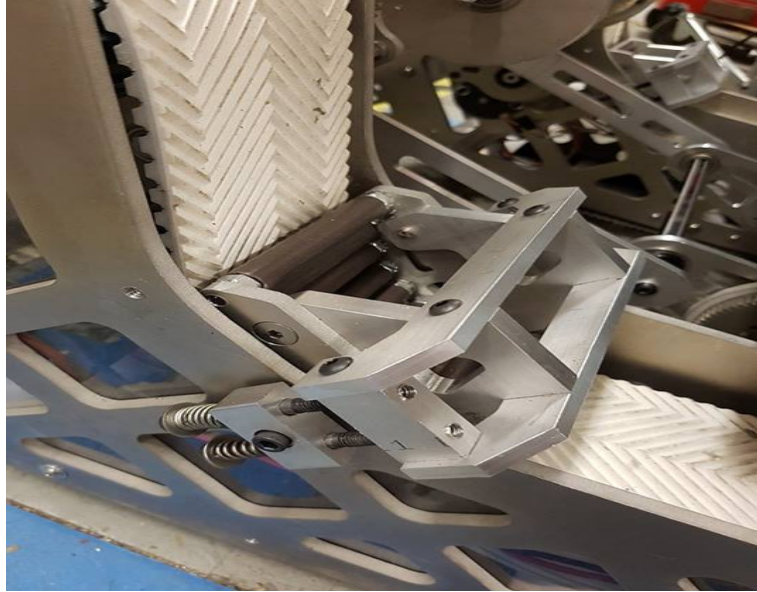
Figure 21: Compliant tensioning system on one of the drive modules
