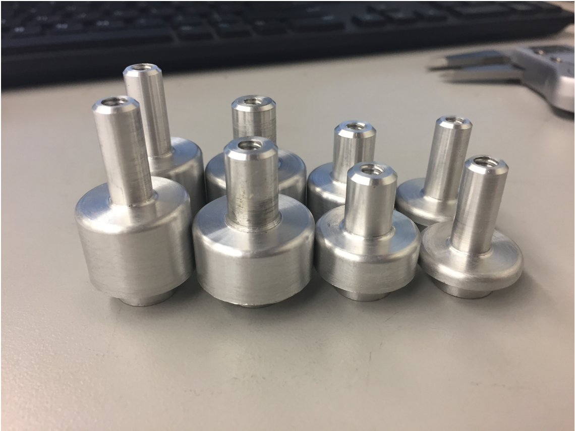
Figure 78: Axles for custom sprockets
