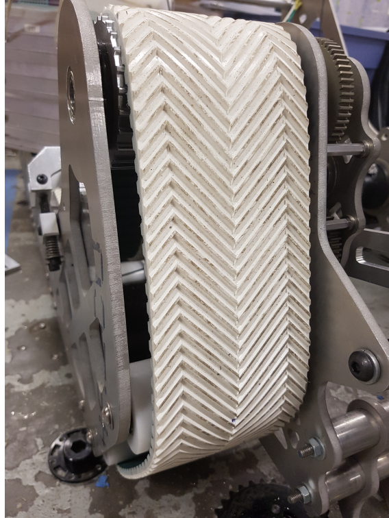
Figure 19: Belt with herringbone pattern
