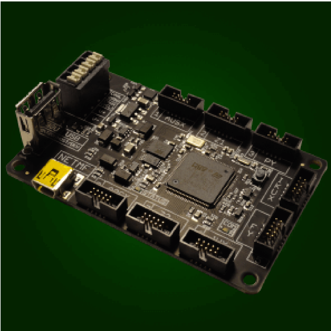
Figure 51: HERO Development Board from Cross the Road Electronics
