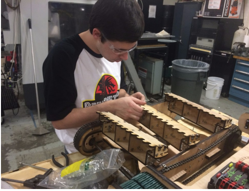
Figure 13: Early models of the collection scoops
