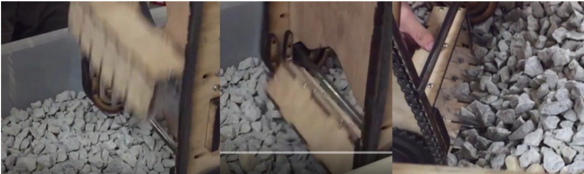
Figure 36: Entering, disturbing, and pushing gravel
