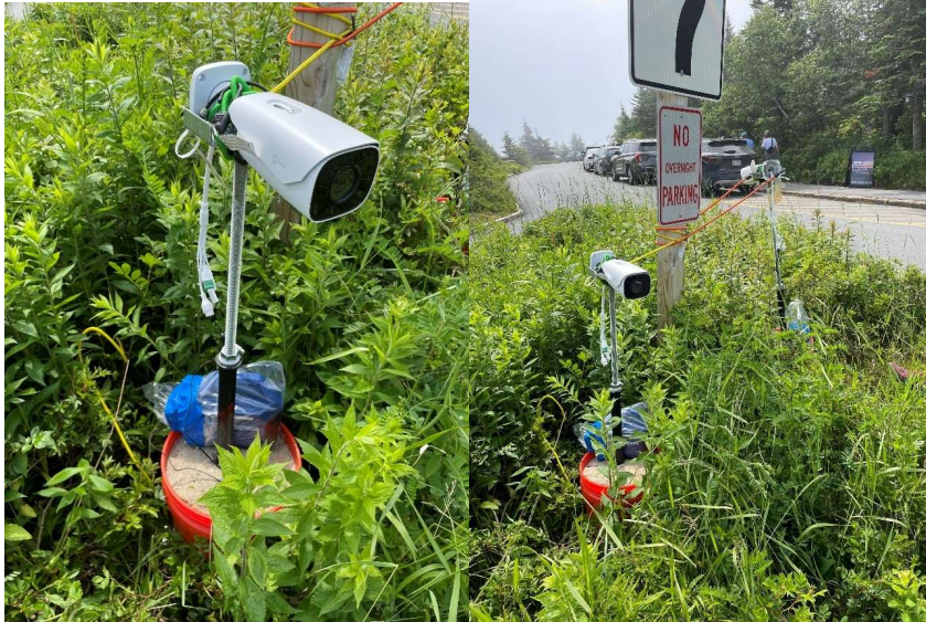
FIGURE 2: LICENSE PLATE READERS SETUP AT THE SUMMIT OF CADILLAC MOUNTAIN
