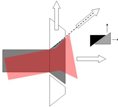
**Figure 6.6** Screw motion due to wedge action
