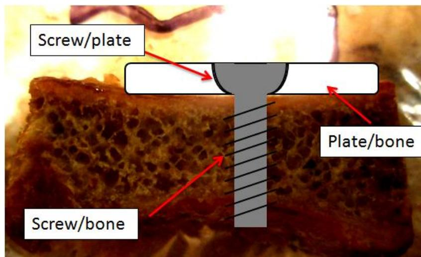
Figure 6.1 Rigid fixation interfaces
