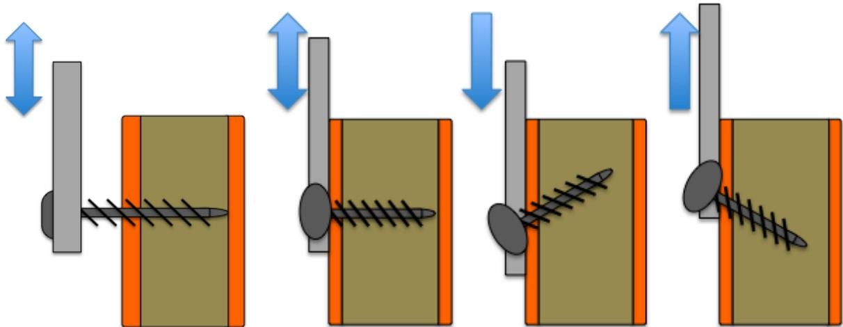
Figure 6.9 Screw pivoting as the mechanism of loosening
