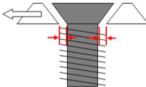
**Figure 6.7** Screw movement due to plate inner diameter
