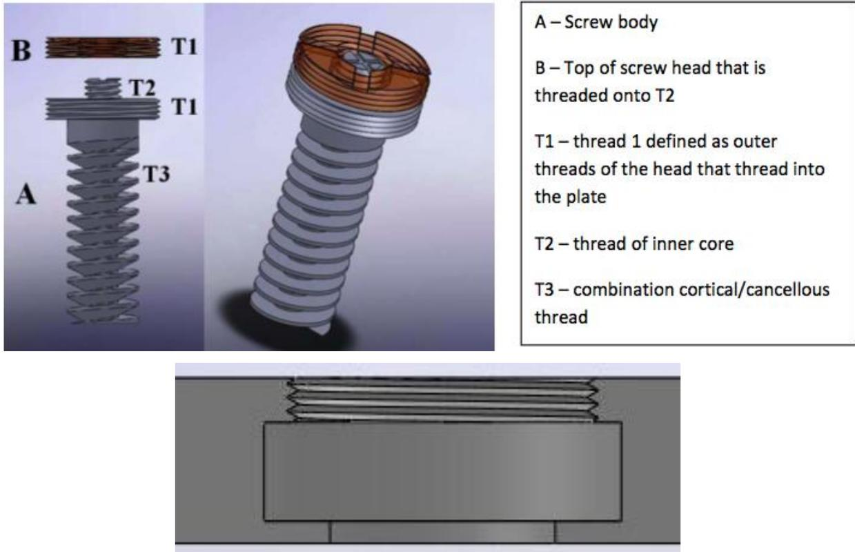
Figure 7.1 Screw component layout and plate design
