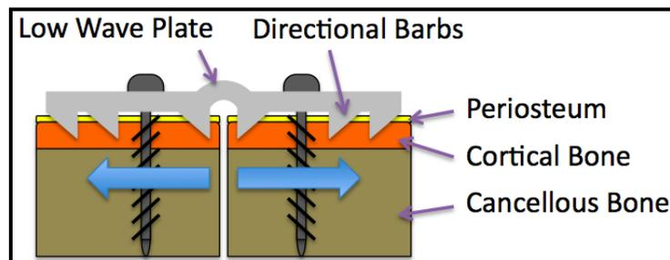
Figure 9.1 Friction wave plate design schematic
