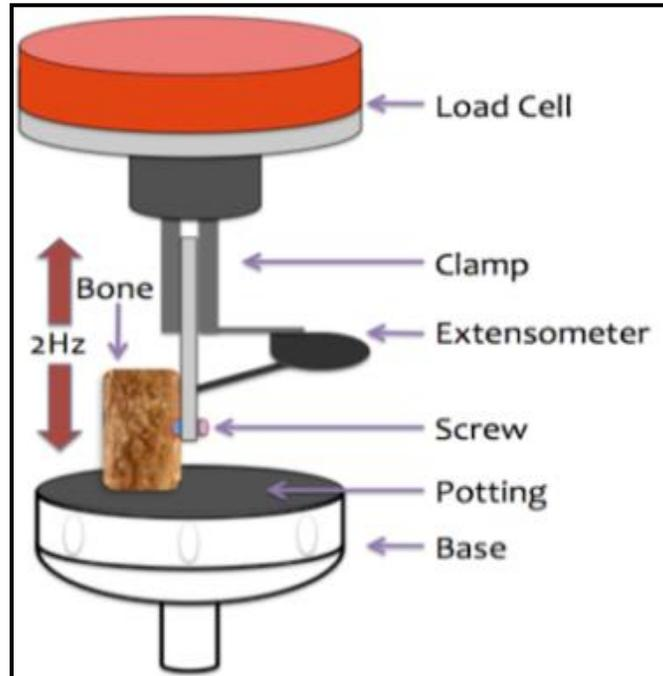
Figure 3.3: Mechanical testing apparatus
