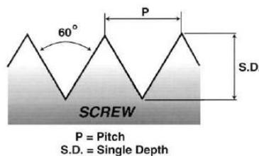
Figure 2.7 Screw Pitch Parameters (An & Draughn, 2000)
