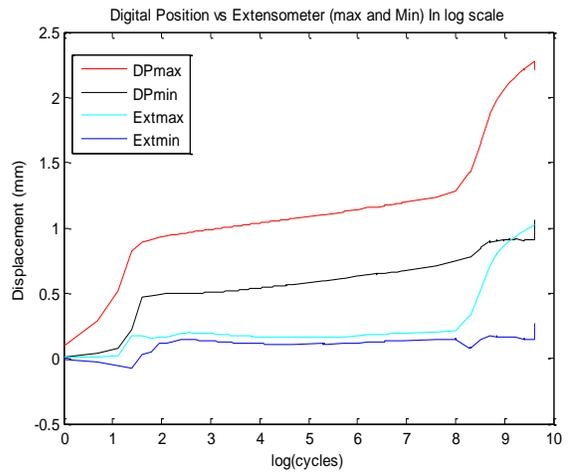
Error: bone sample failed from fixation screws and cement site
