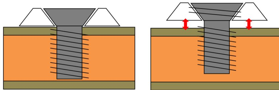
Figure 6.8 Decrease in friction-fit for locking screws
