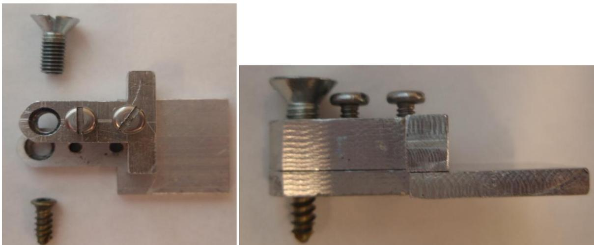
Figure 4.5 Anti-wobble screw-plate system
