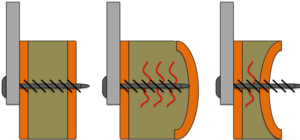
Figure 6.3 Failure modes of bicortical purchase in osteoporotic bone.
