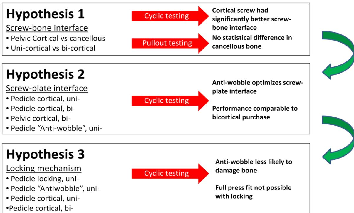
Figure 5.4 Flowchart of Design Verification Steps
