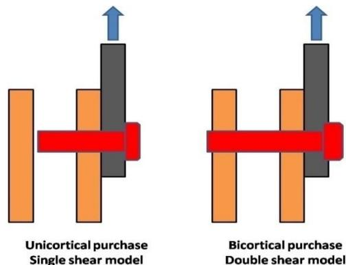
Figure 6.2 Single and double shear models
