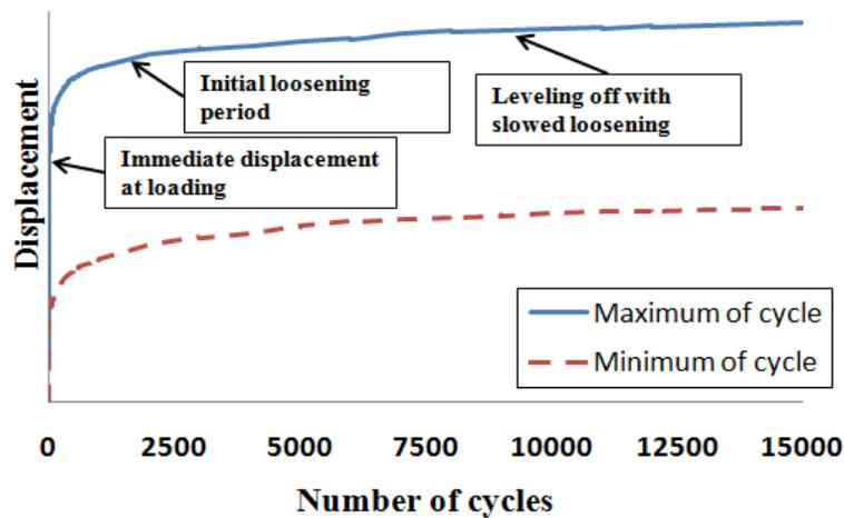
Figure 3.1 Typical displacement curve generated from cyclic loading
