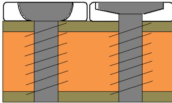
Figure 6.4 Diagram of two head designs: left – orthopedic, right – maxillary-facial
