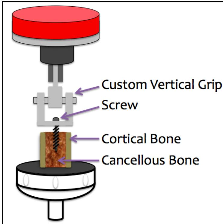
Figure 3.4 Pullout testing apparatus
