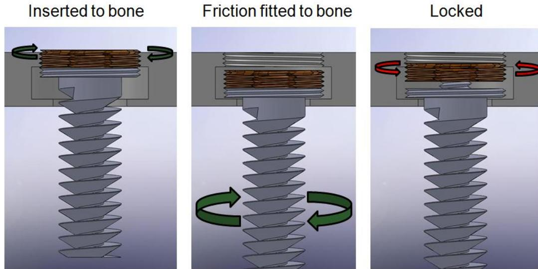
Figure 7.2 Final design method of toggling between non-locking and locking
