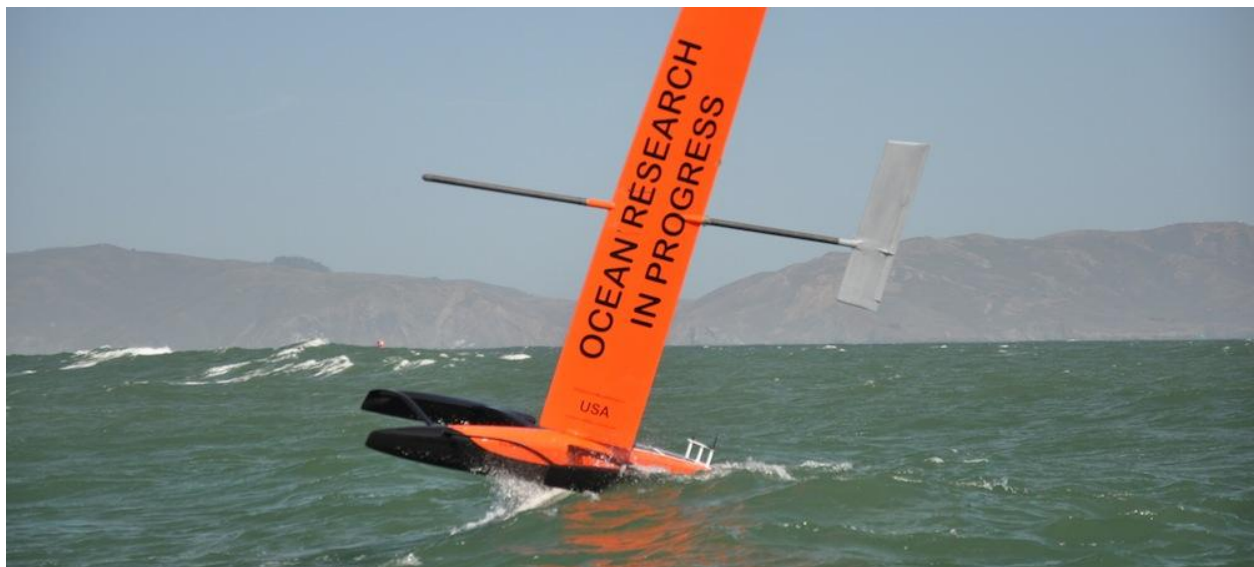
Figure 5: A prototype Saildrone on a test mission ("Saildrone," 2013)
