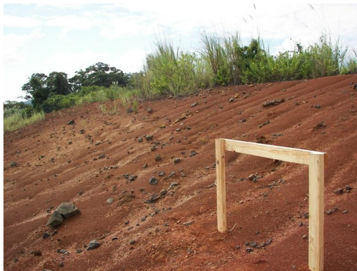
Figure 21 - Soil erosion bridge located at site 6 showing clay, basalt pebbles and rill erosion (Photo Credit: Bryan Lee, 2011)
