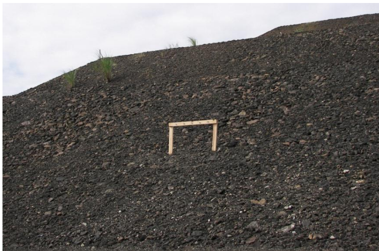
Figure 18 - Soil erosion bridge installed at site 3, with basalt rocks and scattered plant growth (Photo Credit: Bryan Lee, 2011)
