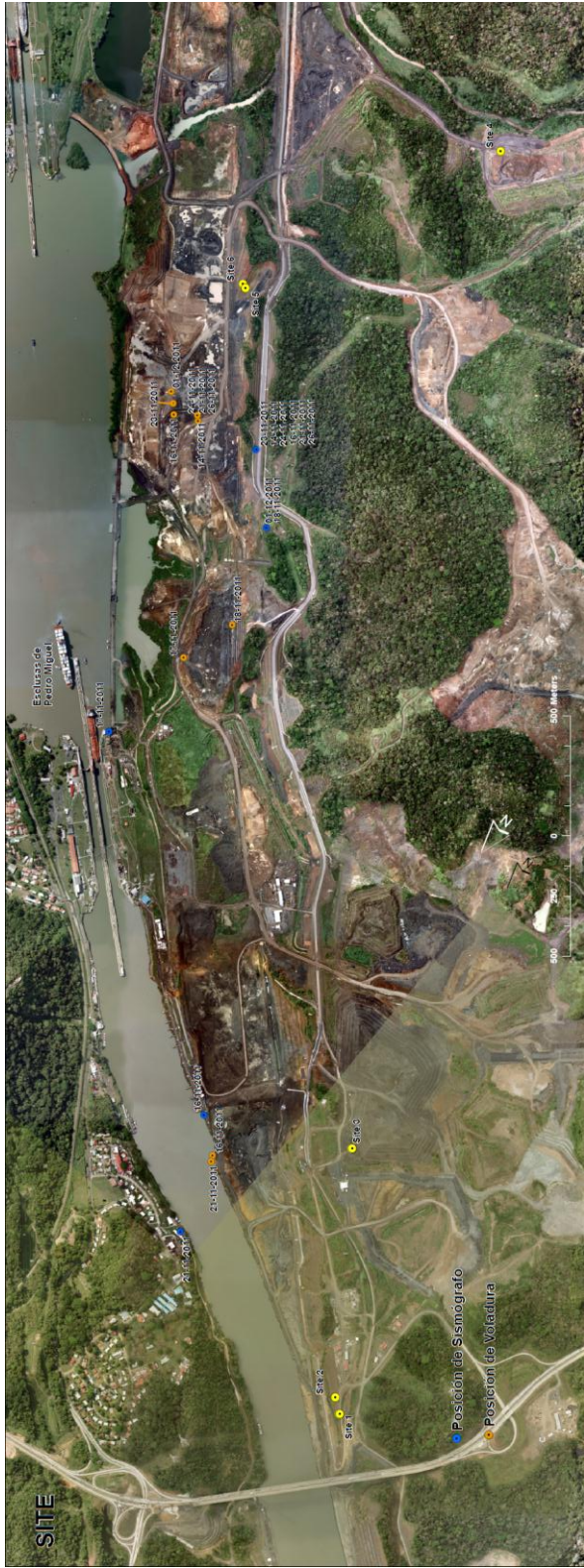
Figure H-1 - GIS map showing blasting locations (yellow dots) and monitoring stations (blue dots)
