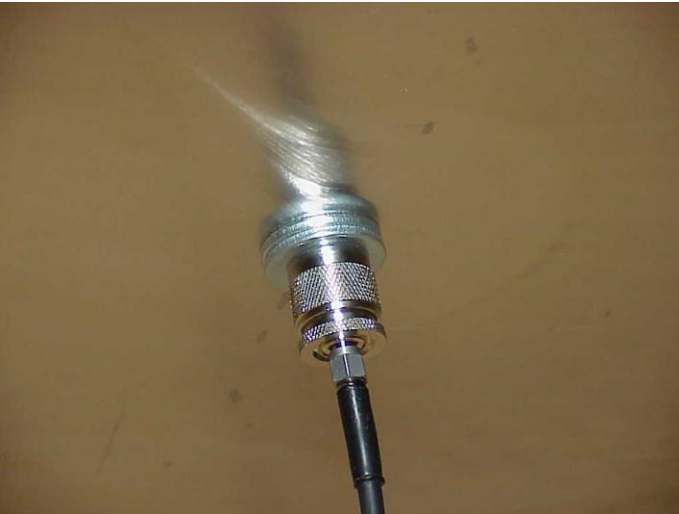
Fig. 17. Antenna feed underneath the ground plane, SMA-to-N-type adapter.
