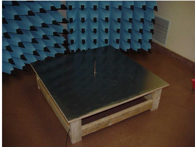
Fig. 14. Blade monopole and 1x1(m) ground plane
