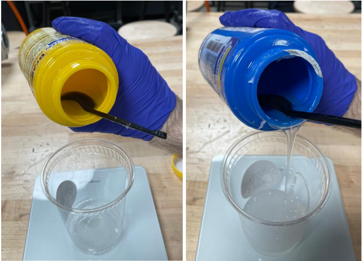
Figure 40: Part A (left) and part B (right) of liquid silicone.
