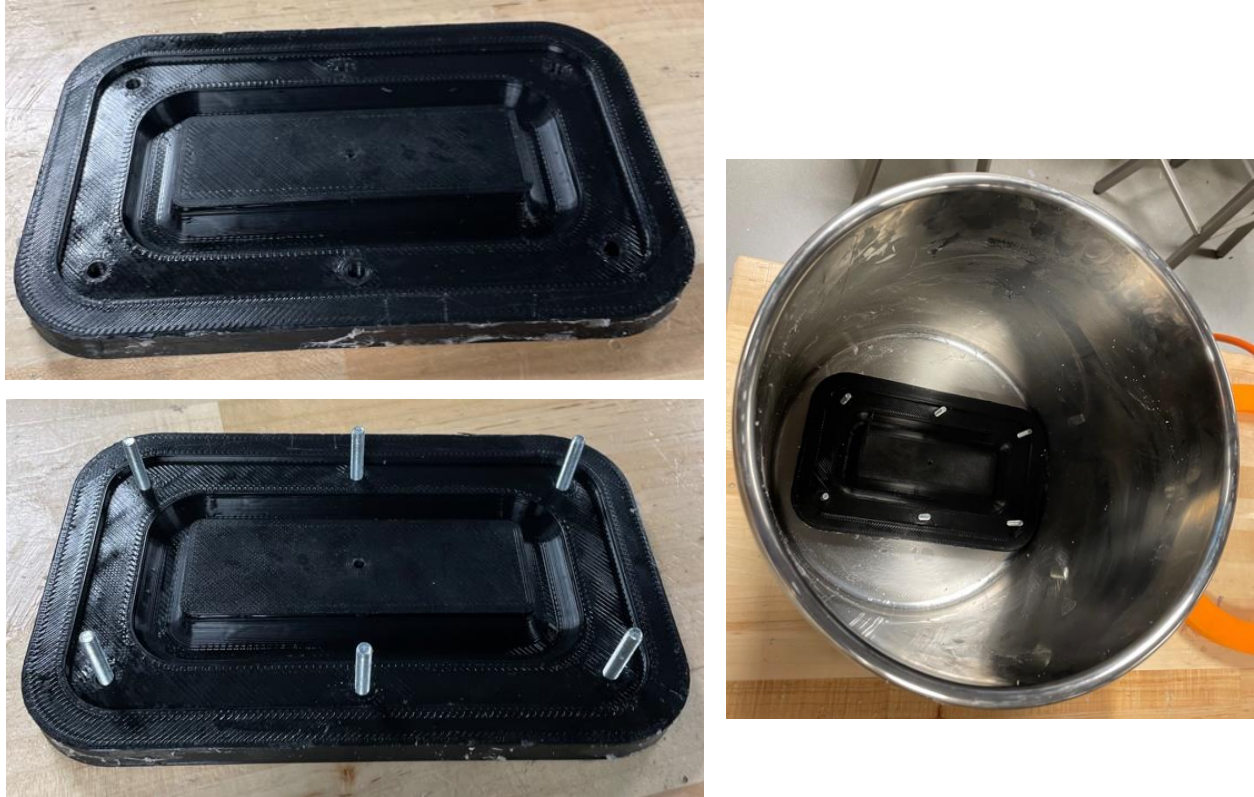
Figure 41: Mold with inserted center piece (top left), mold with inserted center piece and screws (bottom left), mold inside vacuum chamber (right).
