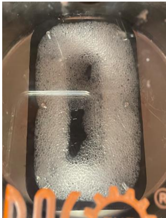
Figure 43: Air being removed from the silicone mixture.
