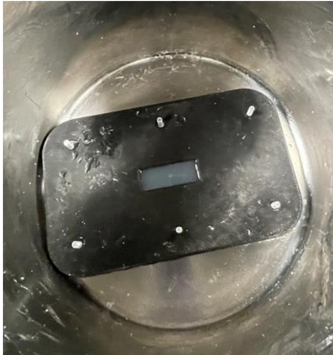
Figure 44: Mold in vacuum chamber with top half added.
