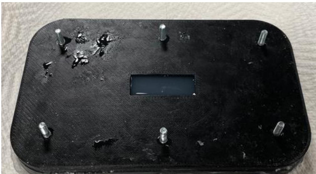
Figure 45: Mold after being removed from the vacuum chamber.
