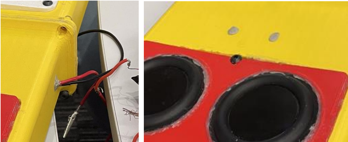
Figure 6: Putty sealing holes for actuator wires and unused actuator mounting holes
