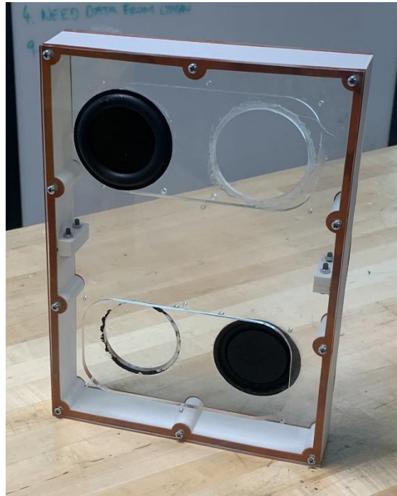
Figure 27: Iteration 1 acrylic speaker. This was never fully assembled as it used iteration 1 active cones.
