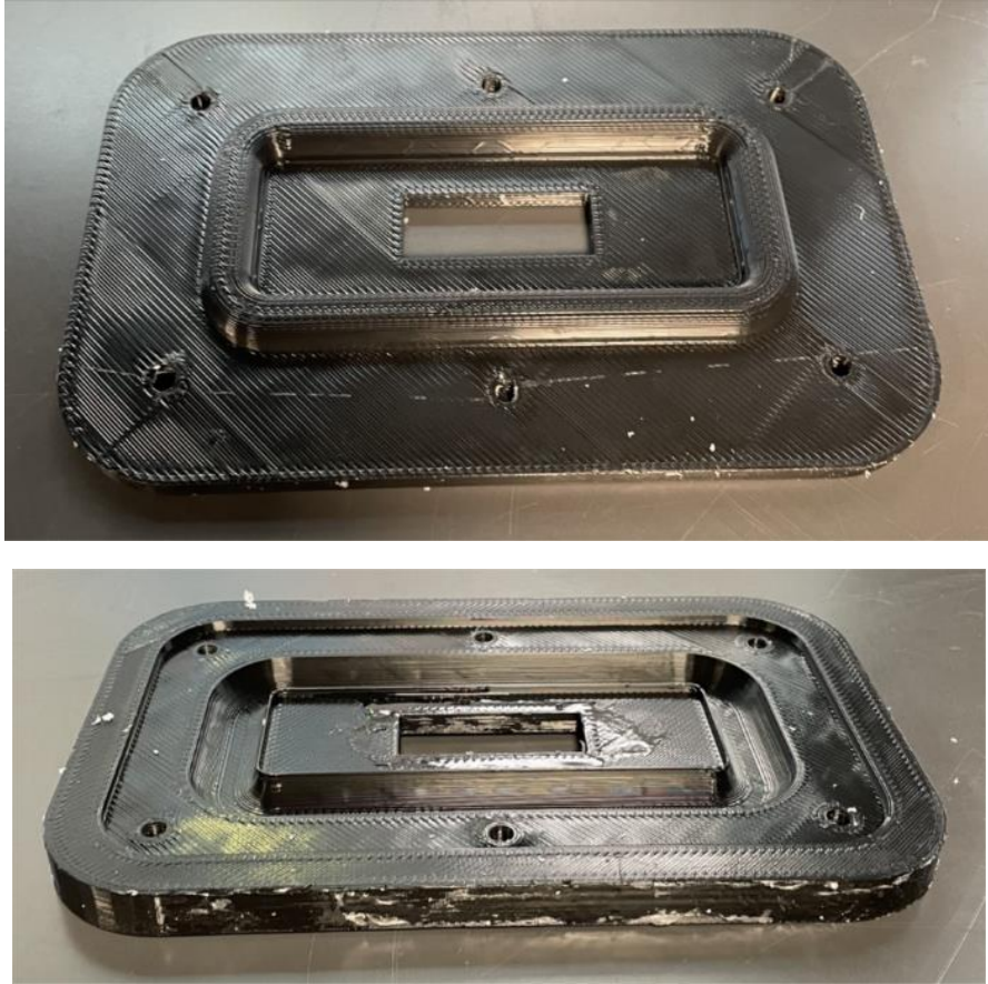
Figure 38: Top half of the mold (top) and bottom half of the mold (bottom).
