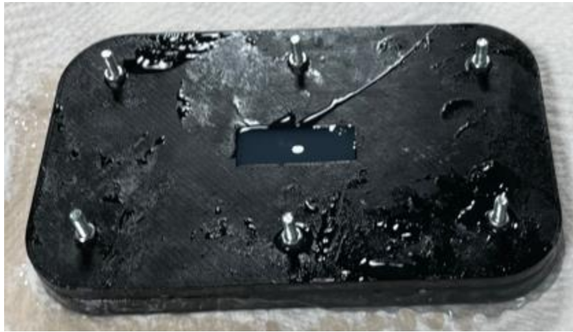
Figure 46: Mold with nuts added to screws.
