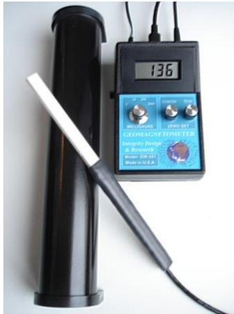
*Figure 7.1: IDR-321 Geomagnetometer with Hall Probe, pictured with accessory Zero Gauss Chamber*
