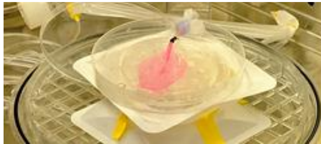
Figure 3-8: hMSC seeded decellularized leaf connected to a hypoxic chamber media perfusion device. A decellularized spinach leaf seeded with hMSCs was placed in a closed-loop elevated perfusion system within a hypoxic chamber. Cell media was perfused through the leaf for 24 hours after which viability was measured.
