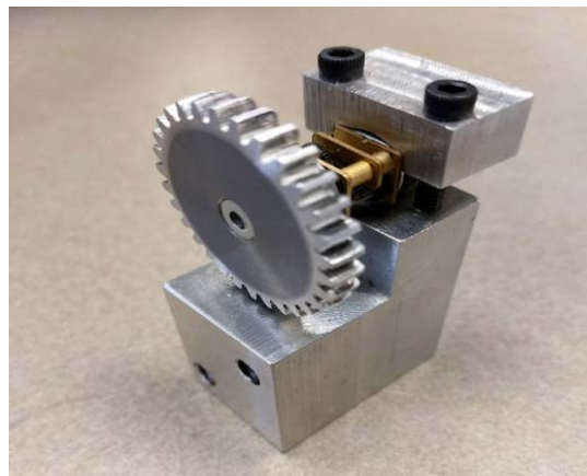
Figure 47: Motor in the Casing
