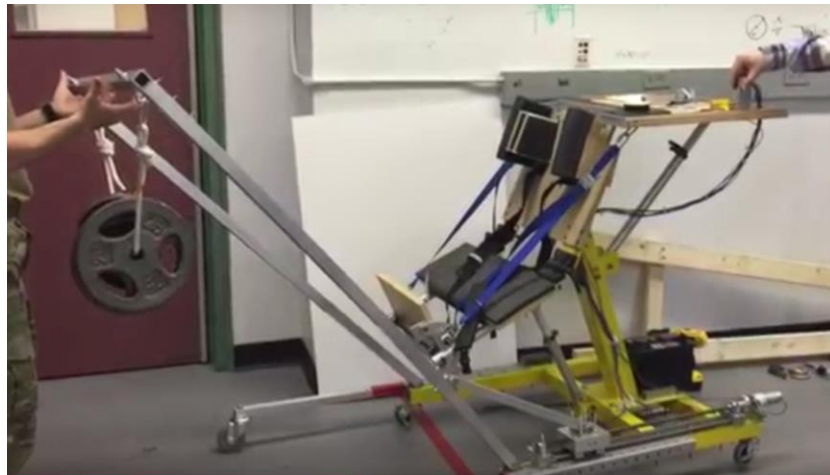
Figure 71 a. Arm Loaded with 75lbs in Position over the Standing Device (Top) b. Arm Loaded with 75lbs in Position over the Wheelchair
