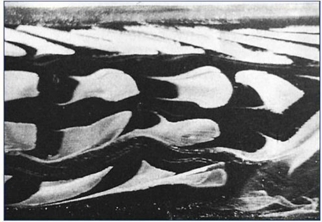
Turbulent flow in a rectangular duct
