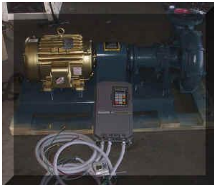
Figure 51: Programmable Sump Pump
