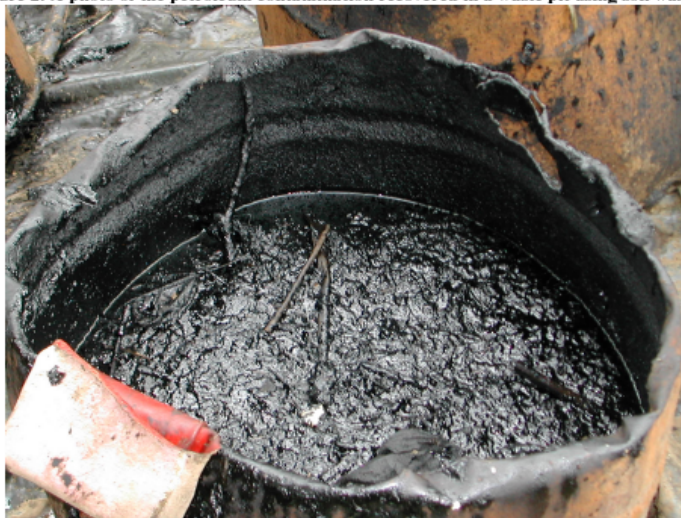
Figure 2: A photo of the petroleum contamination recovered in a waste pit using soil washing.
