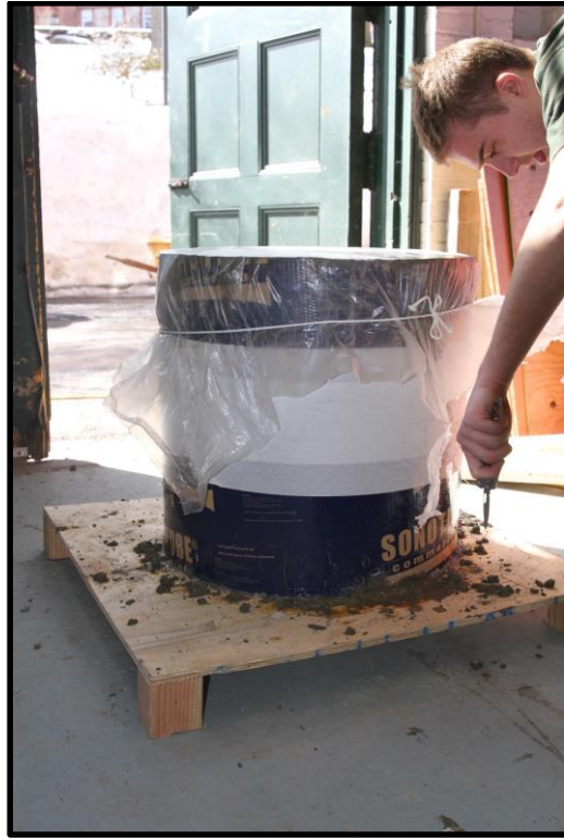
Figure 18: Plastic Covering Mold. From Kaven Hall, Worcester Polytechnic Institute (3/11/2015). Photo by Dan Sanderson.
