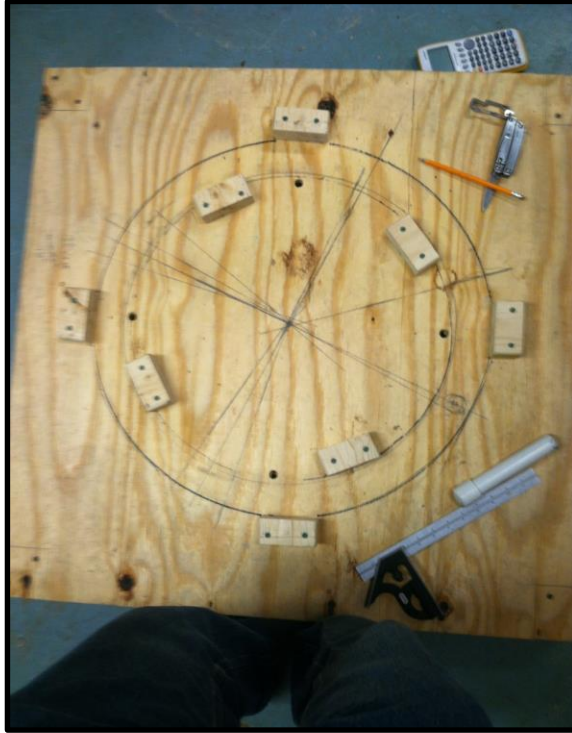
Figure 14: Raised Wooden Platform with Measured Sonotube Placement. (3/8/15)
