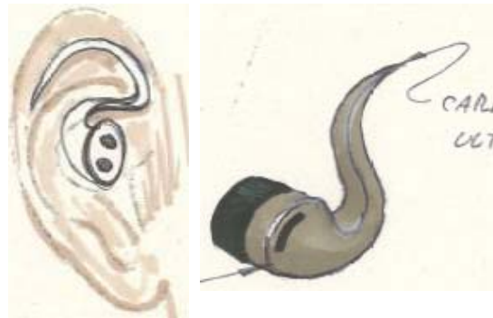
Figure 4.6 - Open Fit Hearing Aid. Shown in the ear (left) and out (right) of the ear
