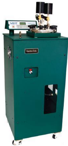
Figure 6: Moisture Induced Stress Test equipment
