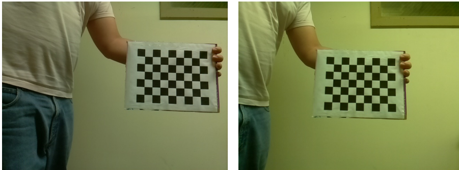
(a) Left and right images of a chessboard pattern taken from a pair of cameras.
