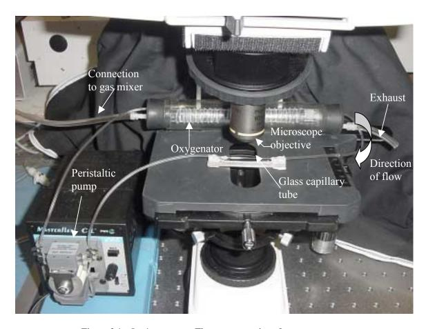
Figure 3.1—In vitro system. The system consists of an oxygenator connected to a gas mixer, a peristaltic pump used for circulating probe solution inside the system, and a square glass capillary tube situated under the microscope objective used for measuring the  $PO_2$  of the solution. The parts are connected with Tygon® microbore tubing, which may be disconnected at various junctions and injected with solution using a 22-gauge needle and syringe.
