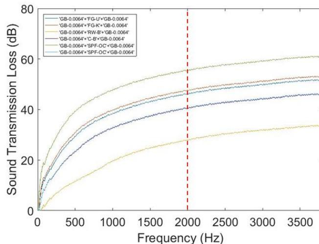
**Figure 35 Sound Transmission Losses of six insulation systems estimated by soundproofing performance sub-model: System number #1 (GB-0.0064m+FG-U+GB-0.0064m), #18 (GB-0.0064m+FG-K+GB-0.0064m), #35 (GB-0.0064m+RW-B+GB-0.0064m), #52 (GB-0.0064m+C-B+GB-0.0064m), #69 (GB-0.0064m+SPF-OC+GB-0.0064m), #103 (GB-0.0064m+SPF-CC+GB-0.0064m)**
