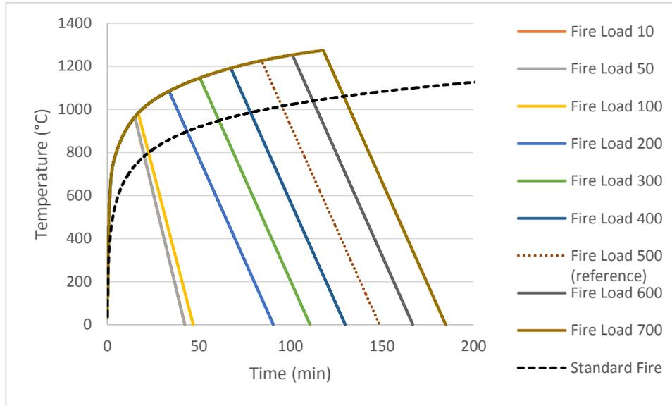
**Figure 50. Time-Temperature curves in EUROCODE by fire load**
