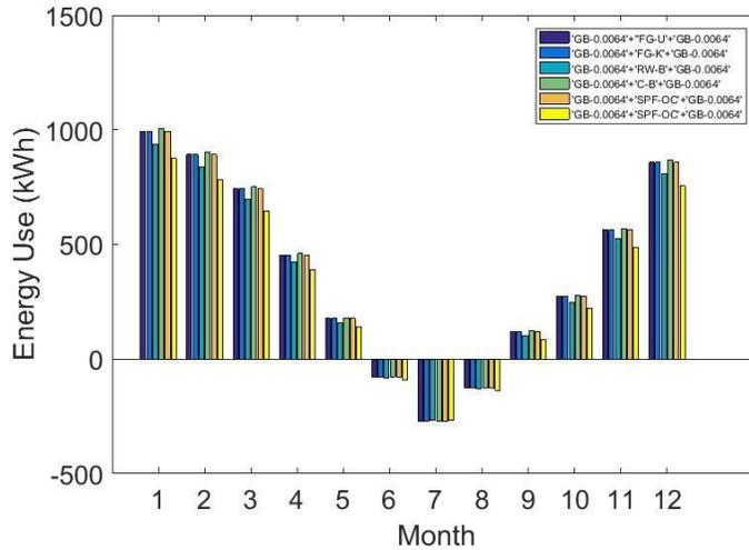
**Figure 34. Examples of monthly energy consumptions estimated by the energy performance sub-model: System number #1 (GB-0.0064m+FG-U+GB-0.0064m), #18 (GB-0.0064m+FG-K+GB-0.0064m), #35 (GB-0.0064m+RW-B+GB-0.0064m), #52 (GB-0.0064m+C-B+GB-0.0064m), #69 (GB-0.0064m+SPF-OC+GB-0.0064m) and #103 (GB-0.0064m+SPF-CC+GB-0.0064m)**
