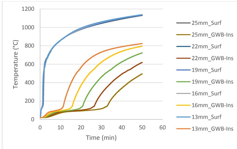
**Figure 60. Heat transfer test results based on the reference fire**
