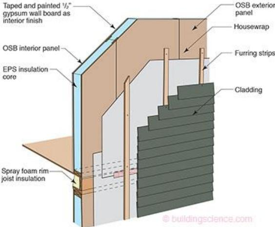
**Figure 45. A wall construed with Structural Insulated Panels [109]**
