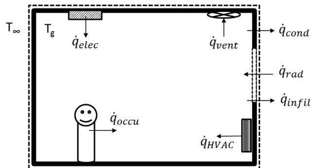
**Figure 11. Schematic diagram for energy balance in the energy performance sub-model**
