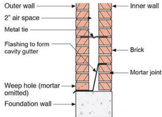
**Figure 42. Masonry cavity walls [105]**
