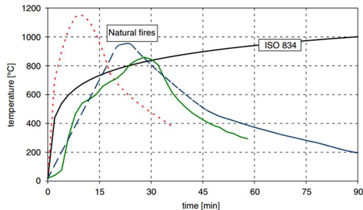
Figure 7. Comparison of temperature-time curves in natural fires with ISO 834 standard fire [40]
