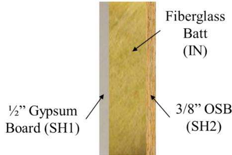
**Figure 37. Reference insulation system**
