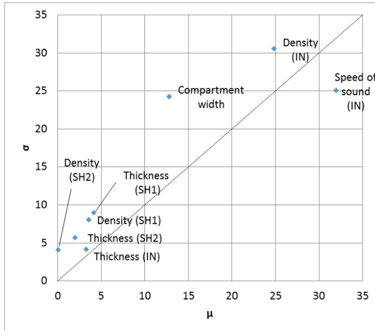
**Figure 23. Results of the sensitivity analysis for the soundproofing performance sub-model on the sound transmission loss**
