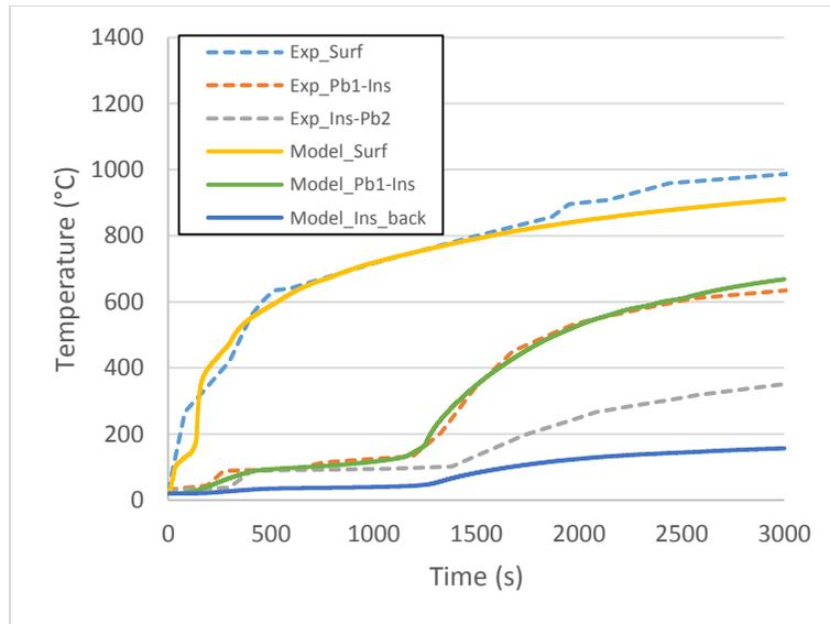
**Figure 58. Temperature profiles of the insulation system of 16mm gypsum board and 32mm glass fiber by experiments and the heat transfer model (Pb1-Ins: the location between gypsum board and the insulation, Ins-Pb2: the location between the insulation and the gypsum board)**
