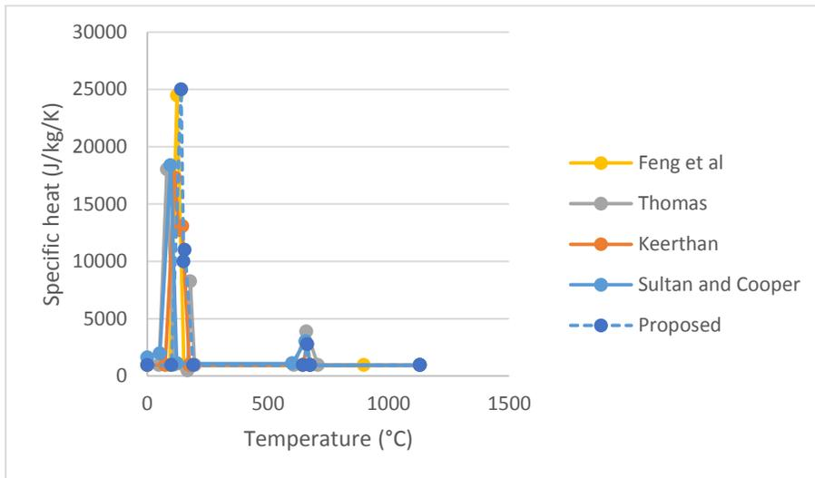
**Figure 18 Specific heats of gypsum boards at different temperatures in various references**
