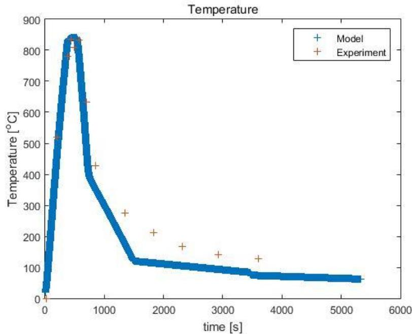
**Figure 53. Comparison of fire severity sub-model and experiment (Experiment is test A1 in ref. [113])**
