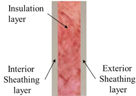
**Figure 1. Insulation system: a layer of insulation, interior and exterior sheathing layers.**
