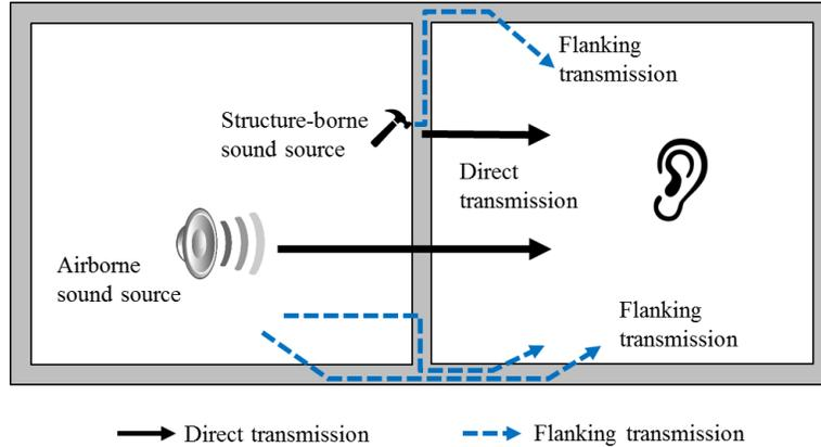
**Figure 3. Sound sources (airborne and structure-borne sound sources) and sound transmission paths (direct and flanking transmissions)**
