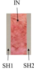
**Figure 20. Insulation system: interior sheathing (SH1), insulation (IN) and exterior sheathing (SH2)**
