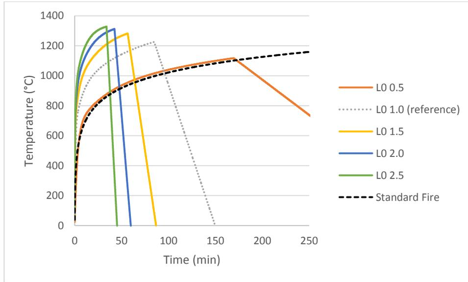
**Figure 48. Time-Temperature curves in EUROCODE by opening length**
