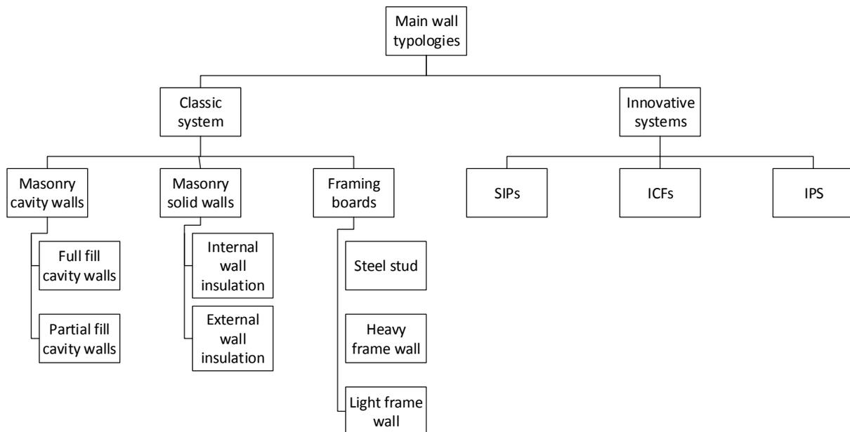
**Figure 41. A schematic diagram of wall typologies for energy efficient buildings (Modified from Hidalgo [50])**
