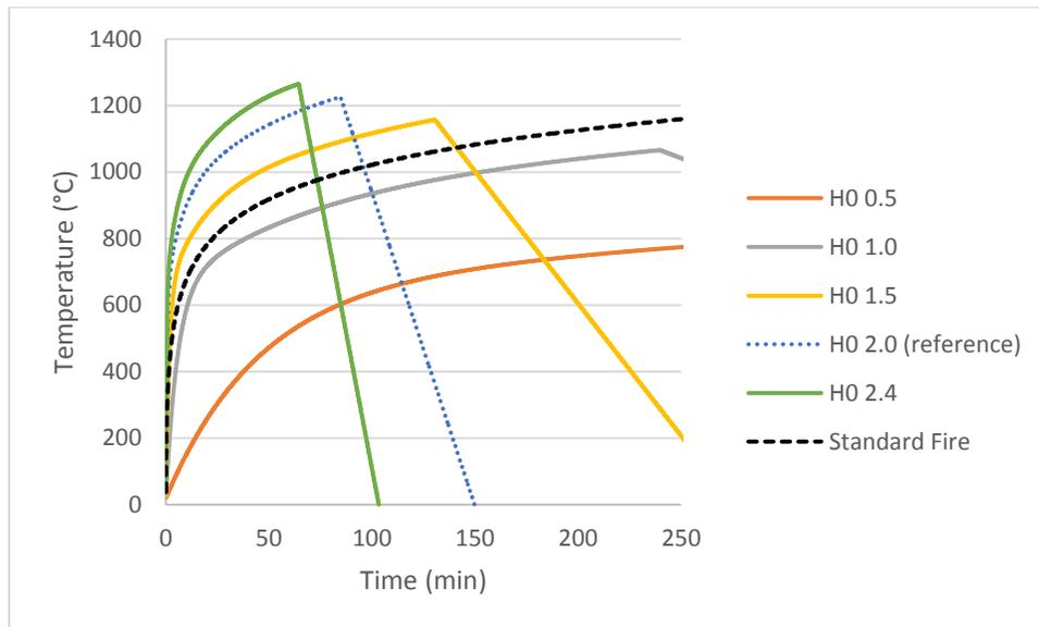
**Figure 49. Time-Temperature curves in EUROCODE by opening height**
