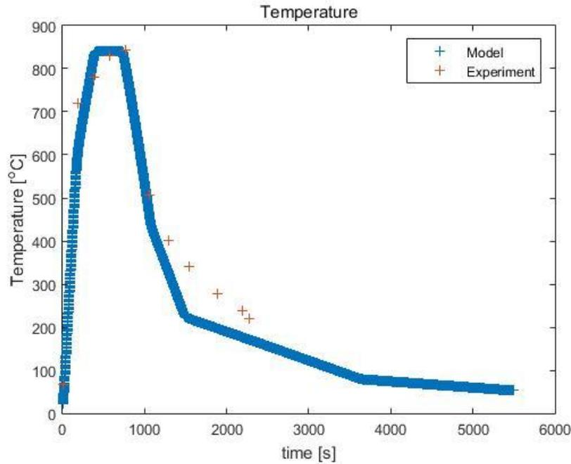
**Figure 54. Comparison of fire severity sub-model and experiment (Experiment is test A2 in ref. [90])**
