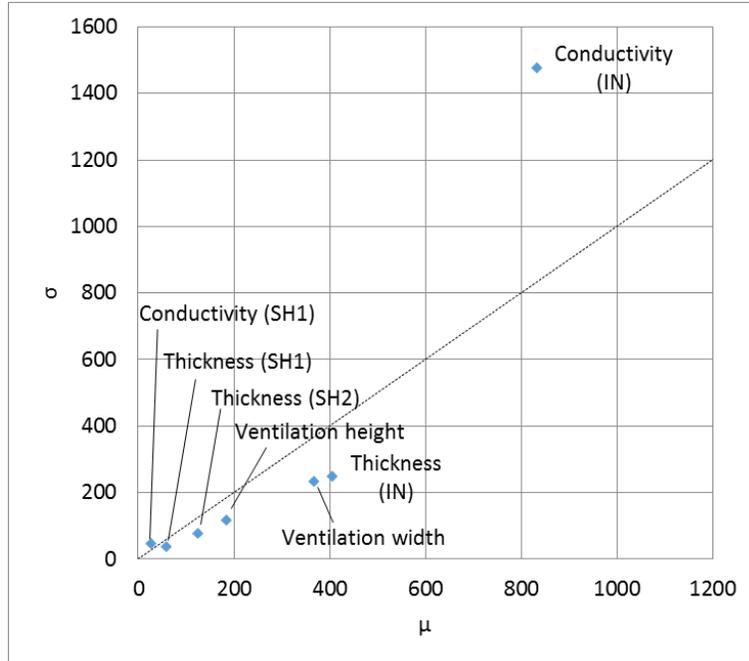
**Figure 22. Results of the sensitivity analysis for the energy performance sub-model on the annual energy consumption**
