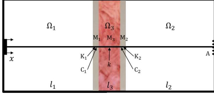
**Figure 13. Schematic diagram of one-dimensional soundproofing performance sub-model:  $x$  is the sound source;  $\Omega_i$  is the acoustic domain, i (e.g. rooms);  $l_i$  is the length of the acoustic domain, i (m);  $M_i$  is mass of the layer (particle);  $K_i$  is the stiffness of the layer;  $C_i$  is the damping coefficient;  $k_i$  is the material propagation constant;  $A$  is admittance ( $\text{m}^3/\text{Ns}$ ) (Figure is modified from reference [65])**
