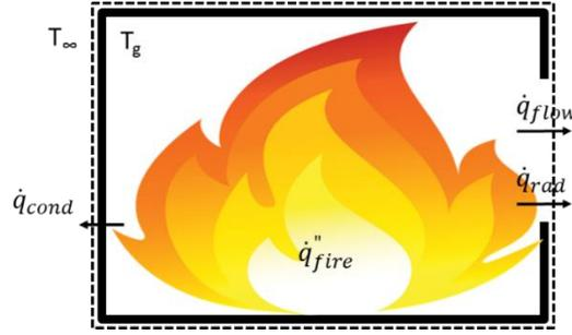
**Figure 12. Energy balance model for the fire severity sub-model**
