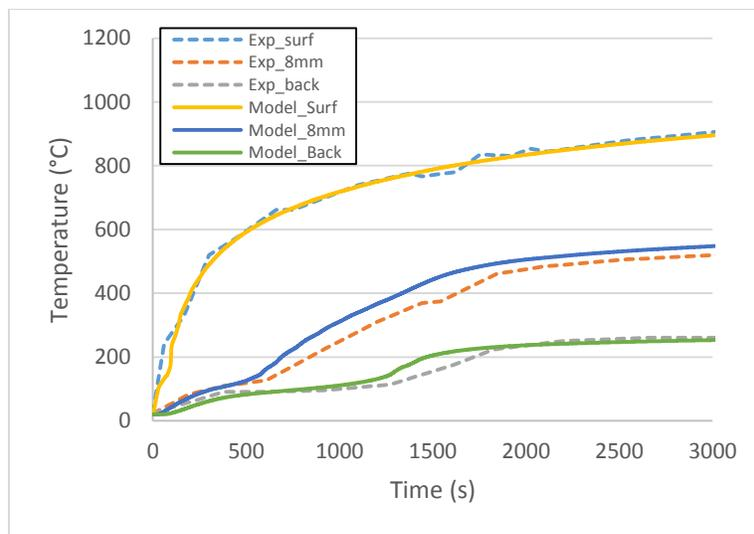
**Figure 57. Temperature profiles for 16mm gypsum board test by experiments and the heat transfer model**
