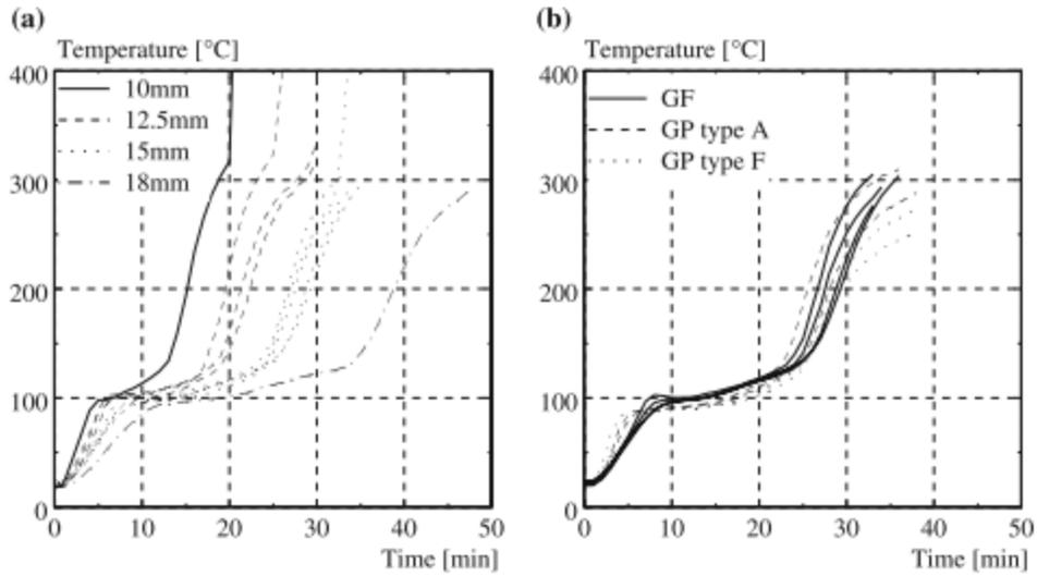
**Figure 15 (a) Temperature development on the fire-unexposed side of gypsum fibreboards of different thickness tested as a single board; (b) temperature development on the fire-unexposed side of different types of 15 mm thick gypsum boards tested as a single board [83].**
