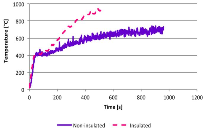
**Figure 5. The gas temperature of heptane fire in the insulated room and non-insulated room [27]**
