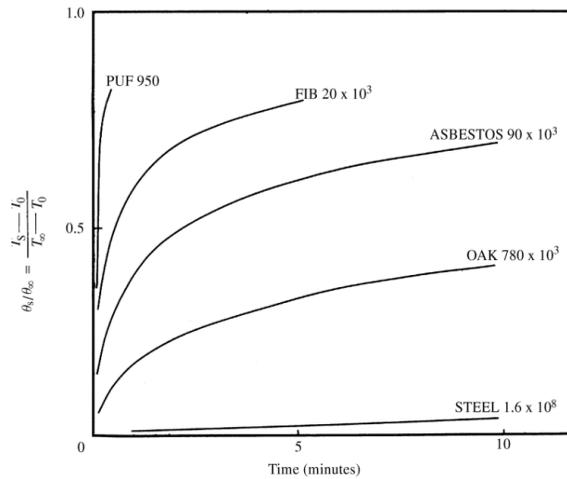
**Figure 4. Effect of thermal inertia on the rate of temperature rise at the surface of a semi-infinite solid PUF (Polyurethane foam), FIB (Fiber Insulating Board) [16]**
