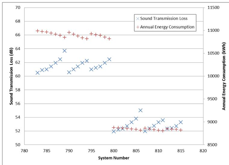
**Figure 40. Soundproofing and energy performance of insulation systems (#783-815)**
