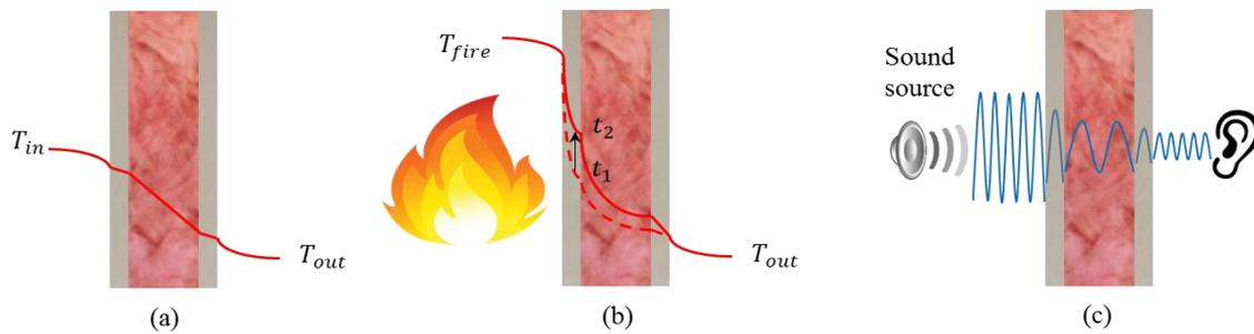
**Figure 2. Three main physical performance of an insulation system: energy performance (a), fire safety performance (b) and soundproofing performance (c)**
