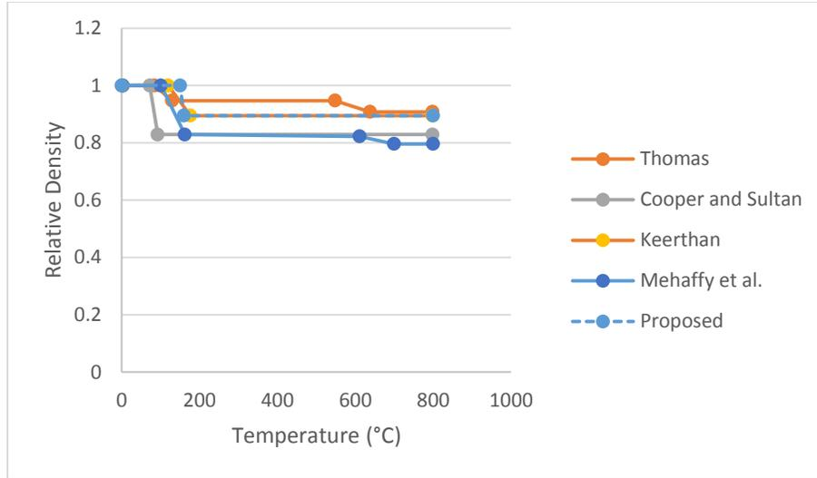
**Figure 19 Relative densities of gypsum boards at different temperatures in various references**
