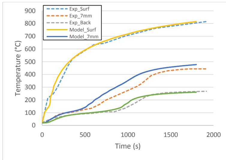
**Figure 56. Temperature profiles for 13mm gypsum board test by experiments and the heat transfer model**
