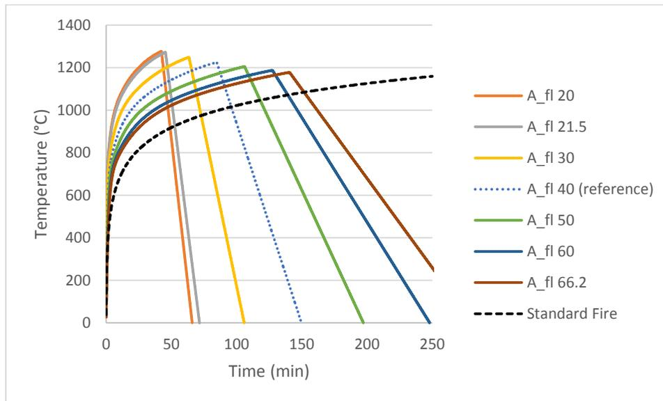
**Figure 47. Time-Temperature curves in EUROCODE by room sizes**
