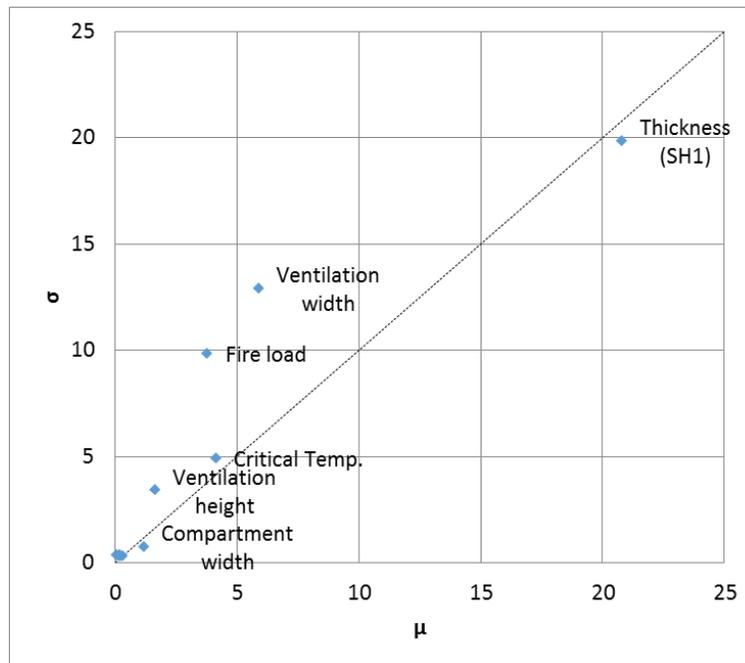
**Figure 21. Results of the sensitivity analysis for the fire safety performance sub-model on the failure time**
