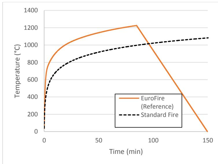
**Figure 59. Reference fire curve by EUROCODE**
