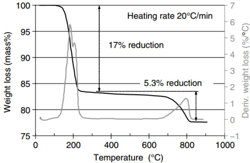
**Figure 16 Curves of the thermogravimetric analysis (TGA) of gypsum in dry air [86]**
