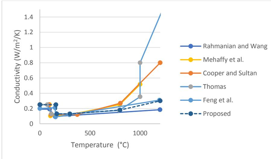
**Figure 17 Conductivities of gypsum boards at different temperatures in various references**
