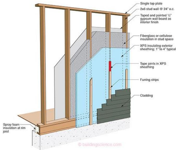
**Figure 43. Wood studs framing walls [107]**
