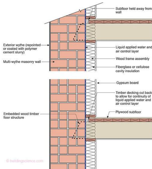
**Figure 44. Masonry solid wall [108]**
