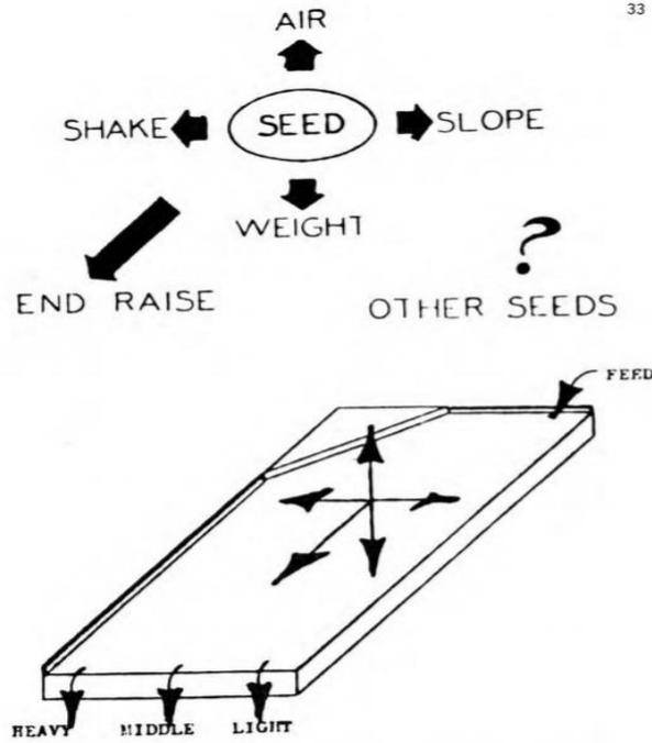
Figure 2: Gravity Table Separation Example and Factors that Influence Separation.
