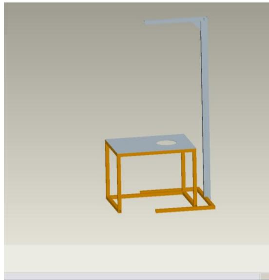
**Figure 20: Cantilever Hoist**
