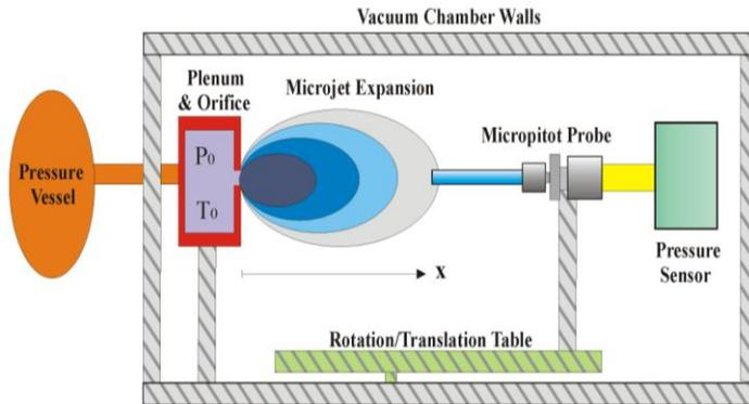
**Figure 1 Experiment Setup from Chamberlin and Gatsonis (2006b)**
