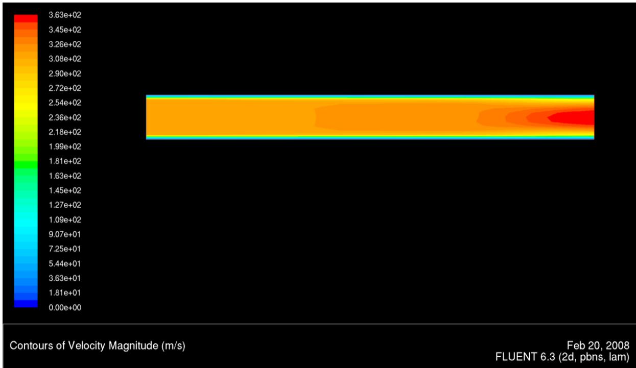
Figure 44 The 10 micron short tube velocity contours
