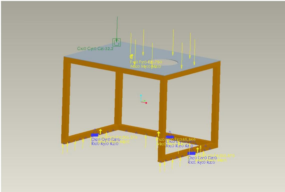
**Figure 5 the table loaded for the analysis**
