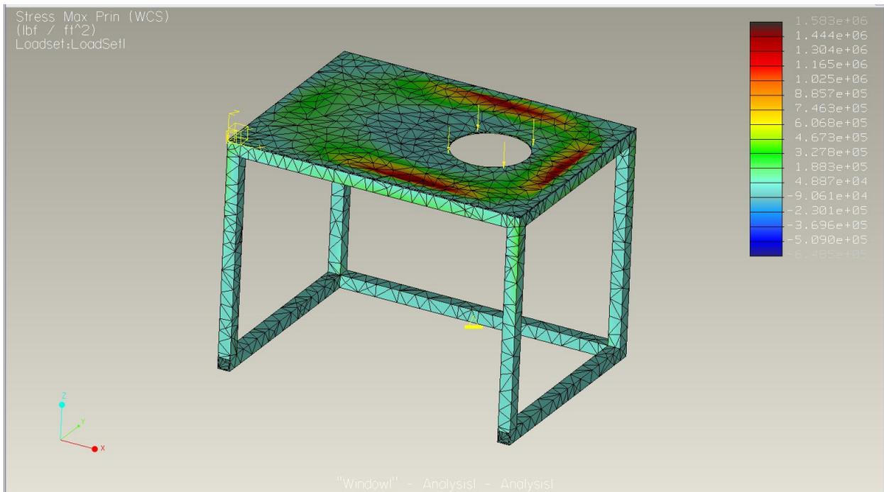
**Figure 7 the Maximum Principle Stress**
