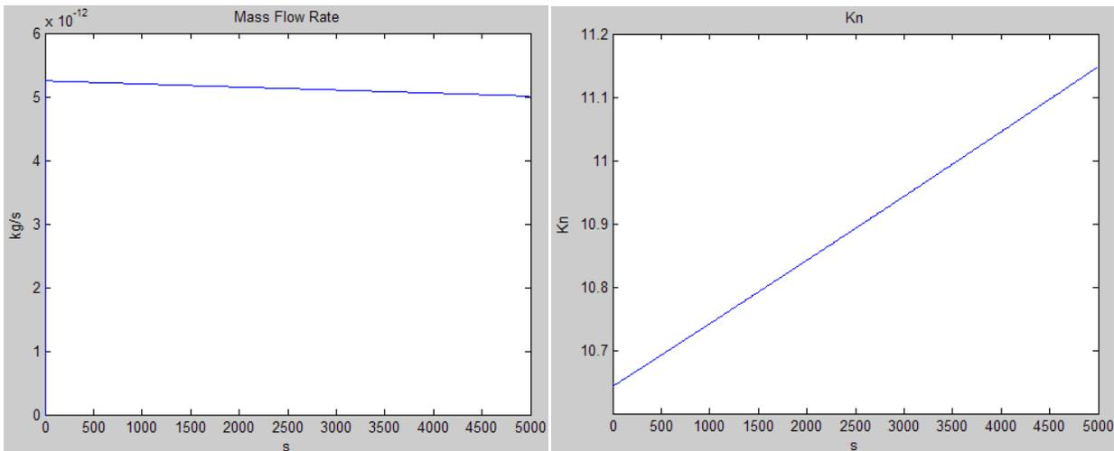
**Figure 38 mass flow and Kn number for the 10 micron tube in free molecular flow**
