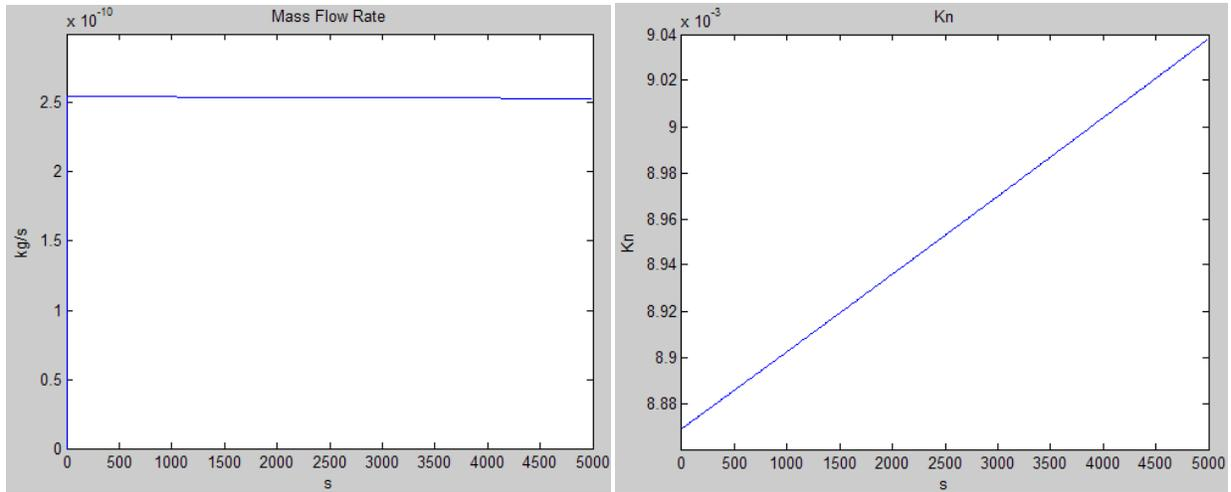
**Figure 33 mass flow and Knudsen number versus time, for the 100 micron continuum flow**
