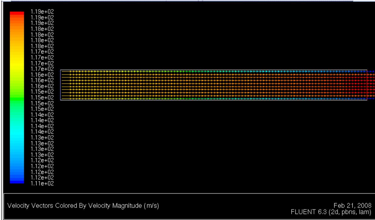
**Figure 42 FLUENT Run for the 100 micron continuum flow (short tube)**
