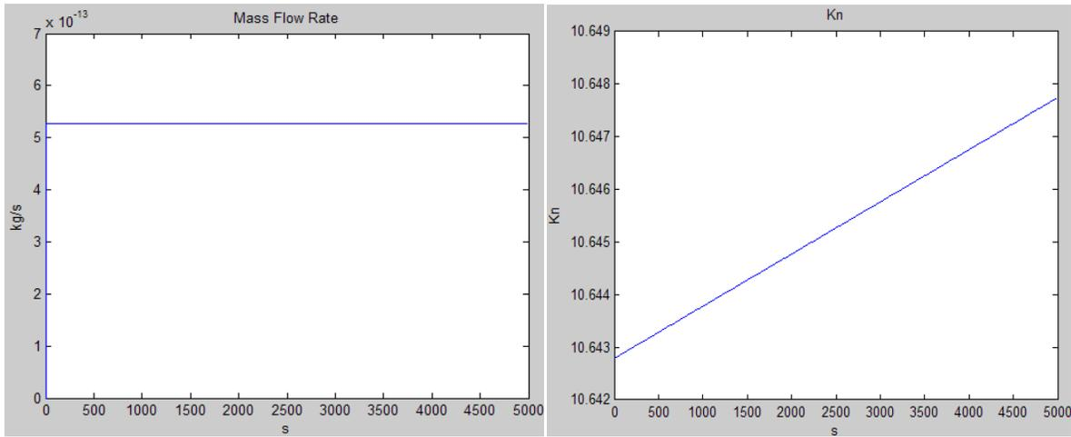
**Figure 41 mass flow and Kn number for a 1 micron tube, free molecular regime**
