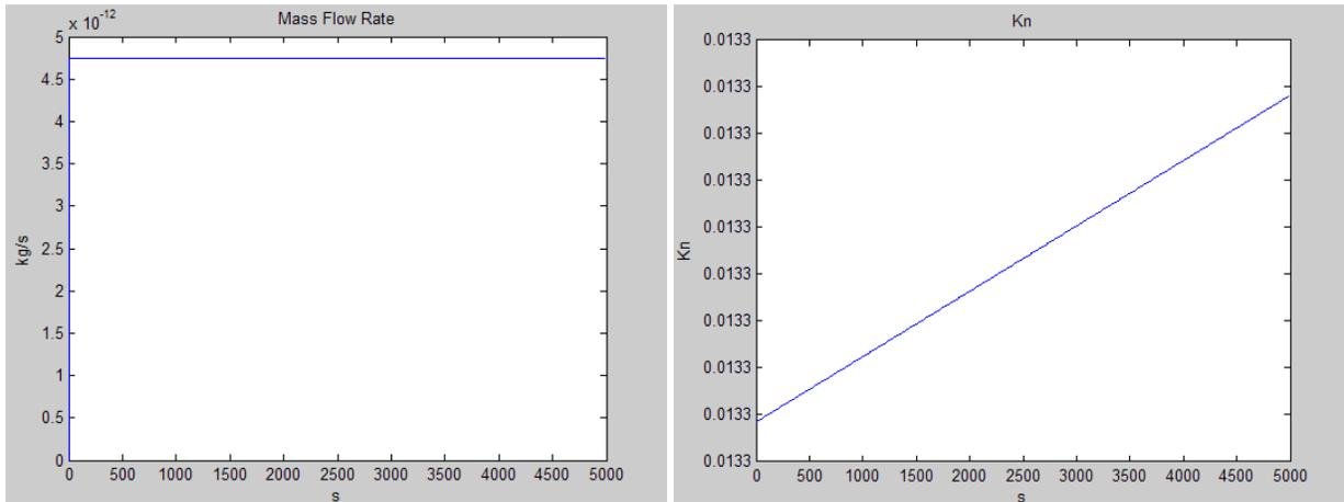
**Figure 37 mass flow and Kn number for 10 micron tube, transitional flow**
