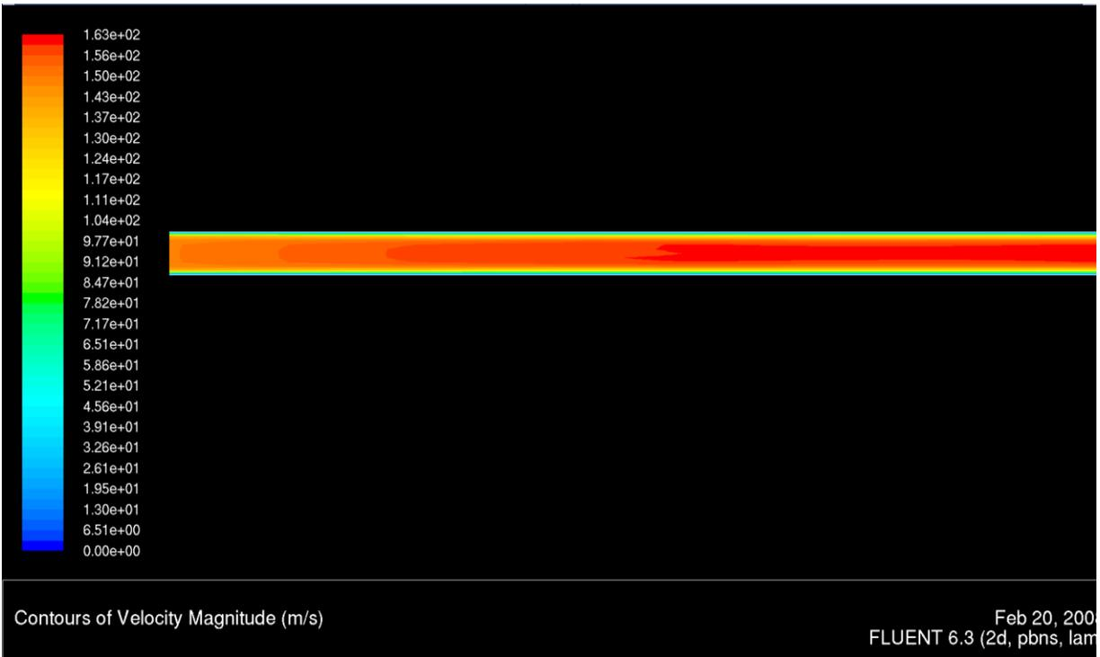
**Figure 43 Velocity Contours for the 10 micron, longer tube**
