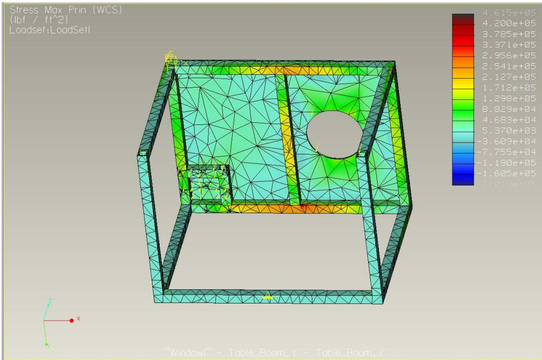
**Figure 29 the bottom view of the max princ.**
