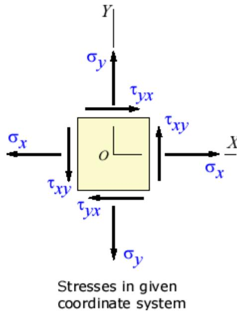
In certain cases, the directions of the stresses ( $x',y',z'$ ) do not line up with the original coordinate set ( $x,y,z$ ):
