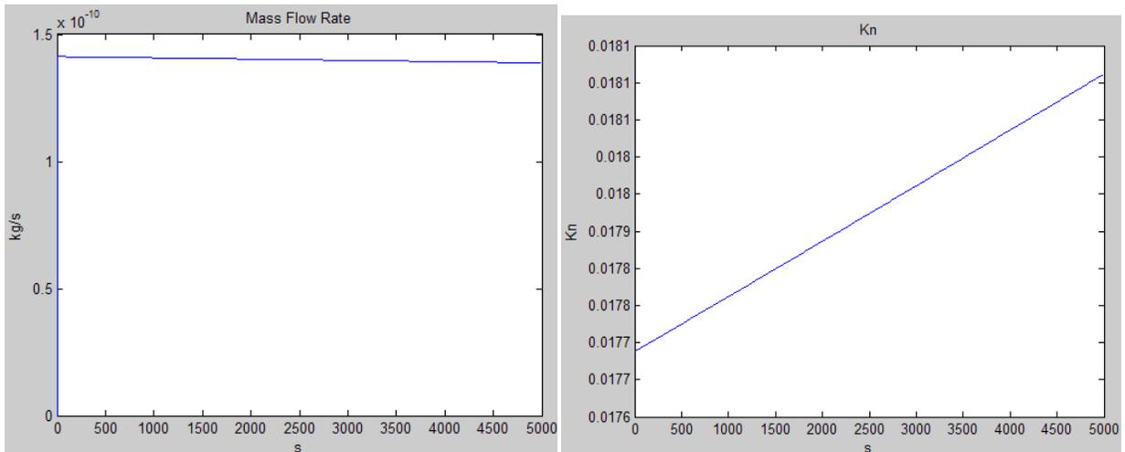
**Figure 34 mass flow and Kn number for 100 micron tube transitional flow.**
