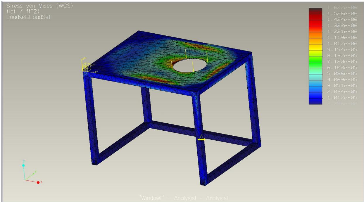
**Figure 6 the Von Mises Results for the offset hole table**
