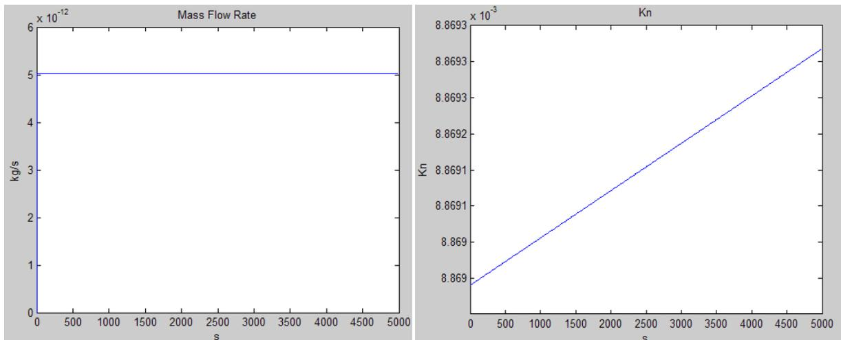
**Figure 36 mass flow and Kn number for 10 micron tube, continuum flow**
