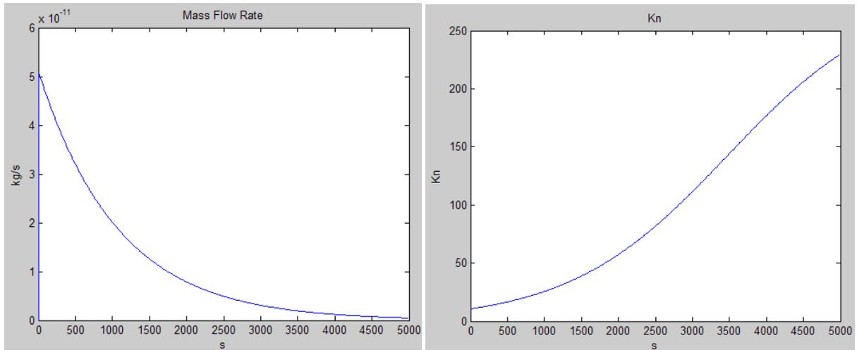
**Figure 35 mass flow and Kn number for a 100 micron tube in free molecular flow**
