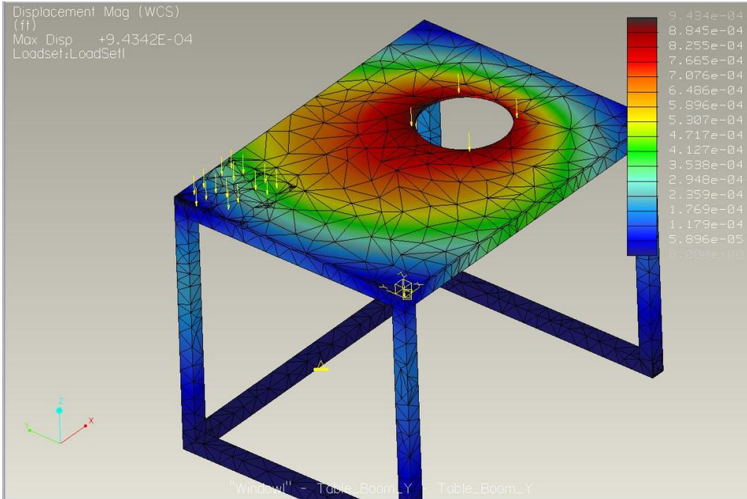
**Figure 30 the Displacement Max=.28mm (9.4342e-4 ft)**
