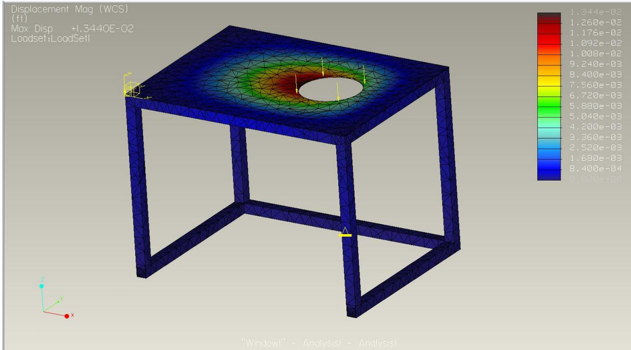
**Figure 8 the Displacement Results (.01344ft=4.09mm)**
