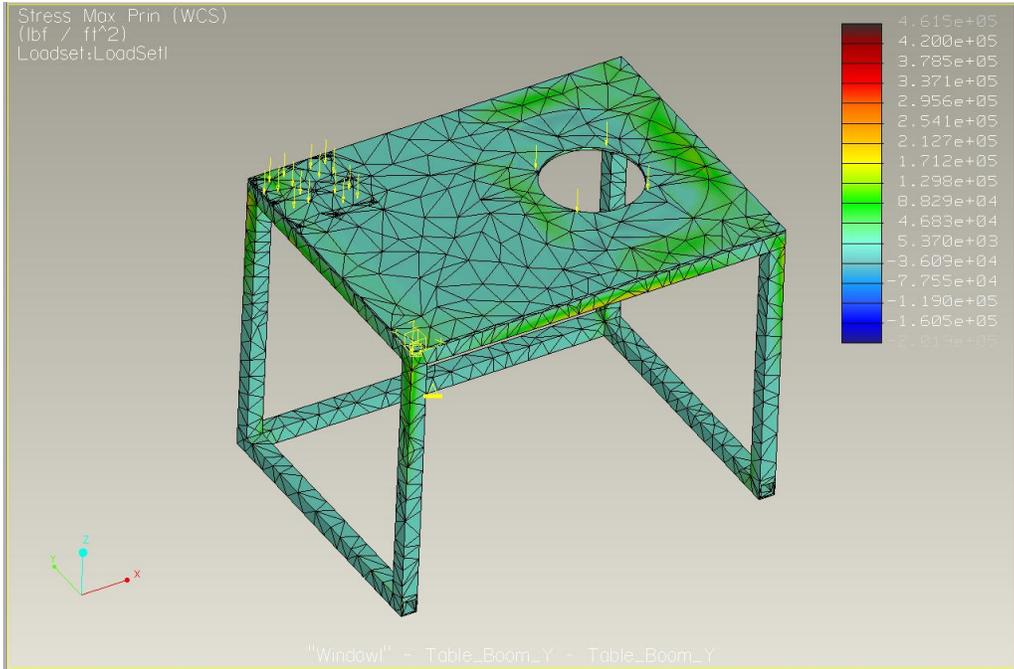
**Figure 28 the Max Princ. Stress results Max= 4.615e5 psf**
