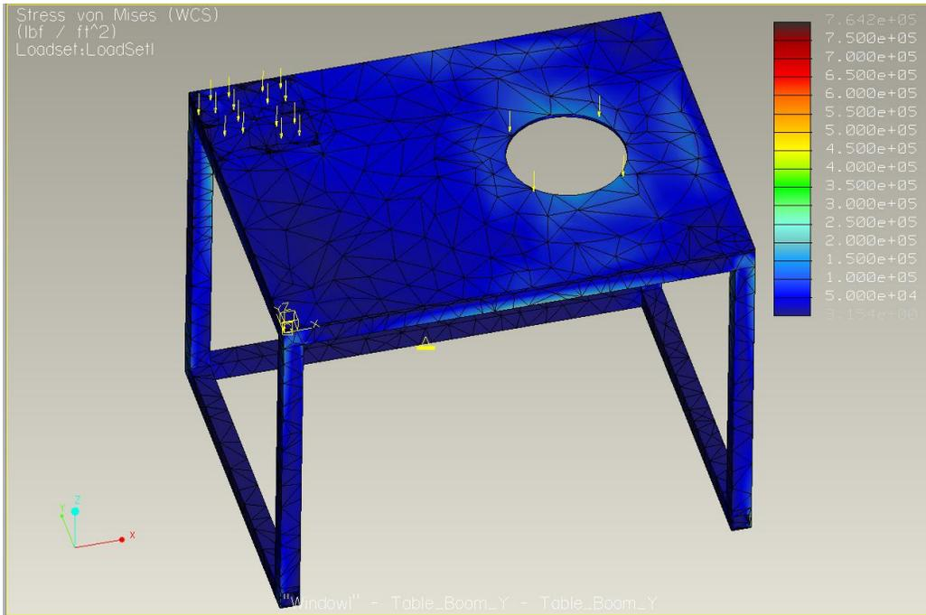
**Figure 26 Von Mises results Max= 7.642e5 psf**
