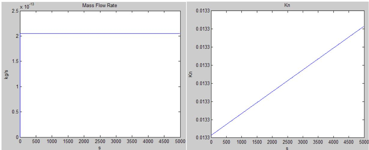
**Figure 40 mass flow and Kn number for 1 micron, transitional flow**
