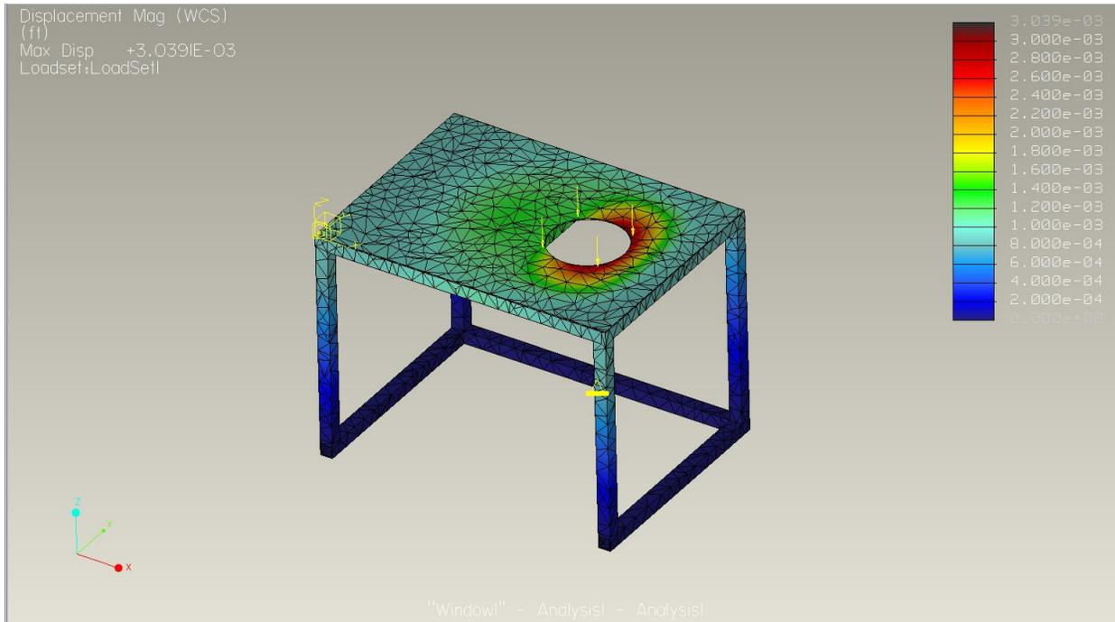
**Figure 9 the displacement results after the cross beam was added (.003ft=.914mm)**
