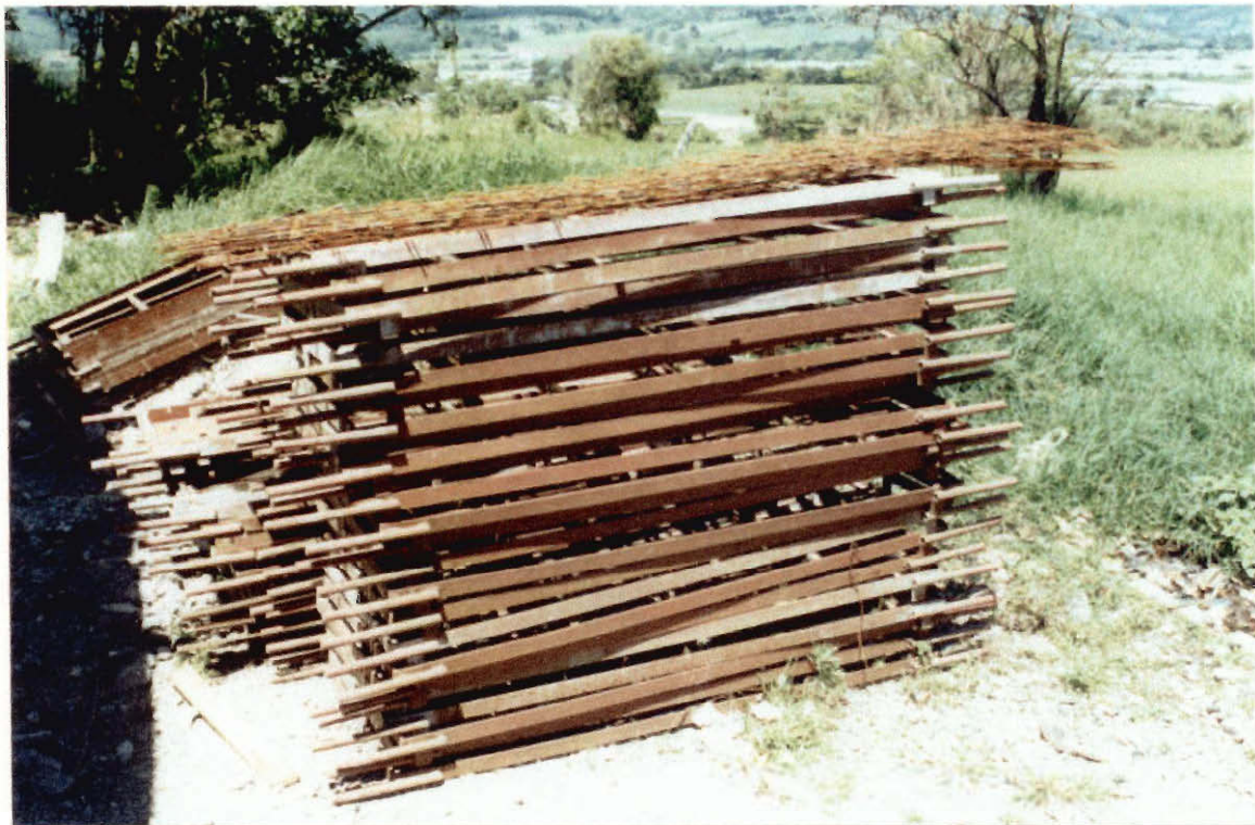
MOLDS USED FOR VIBRATING TABLE
