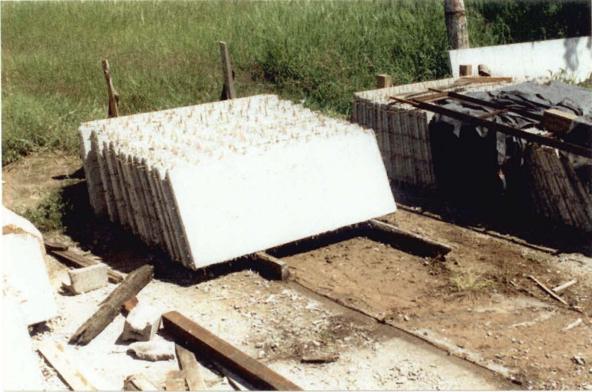
FINISHED HABICON PANELS
