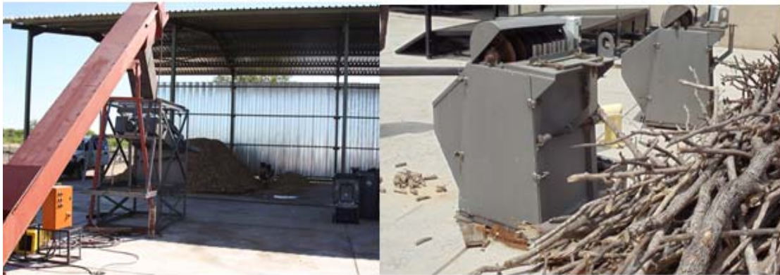
Figure 4.15: The supplied rotatory conveyor (left) and manually-fed cutting table (right)
