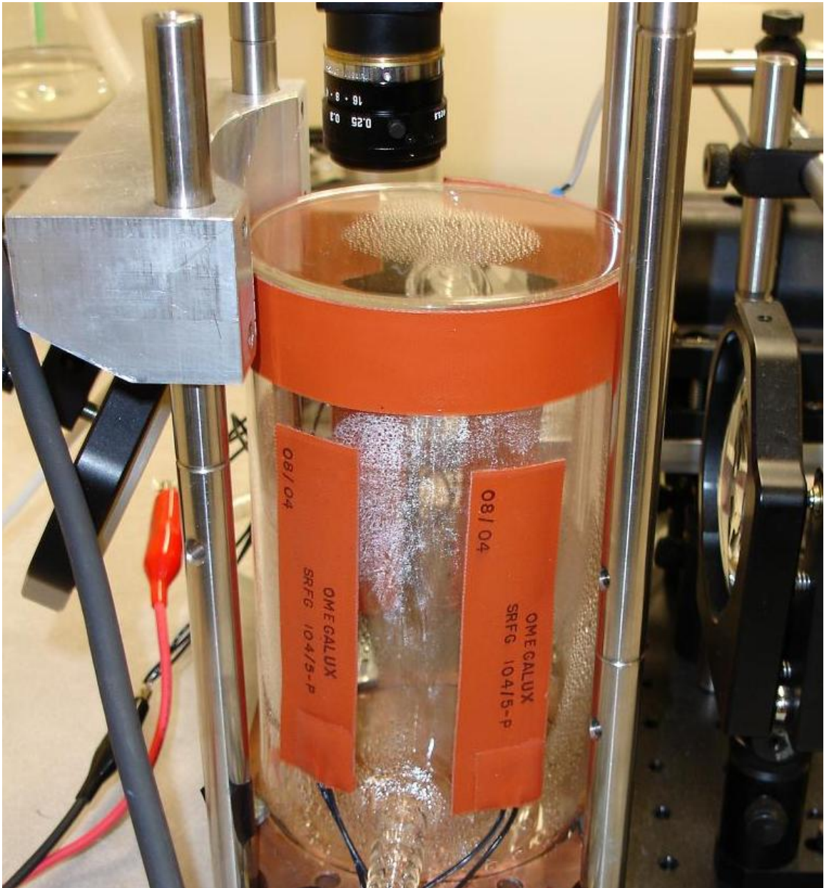
Figure 5-26: Condensation on walls and ceiling of the chamber
