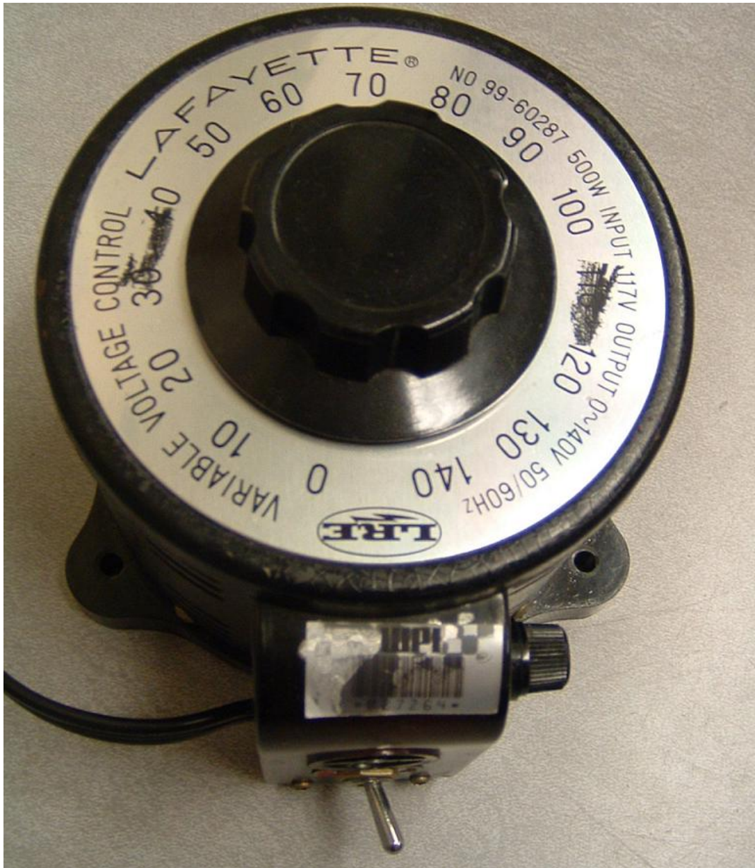
Figure B-7: Variable Voltage Control
