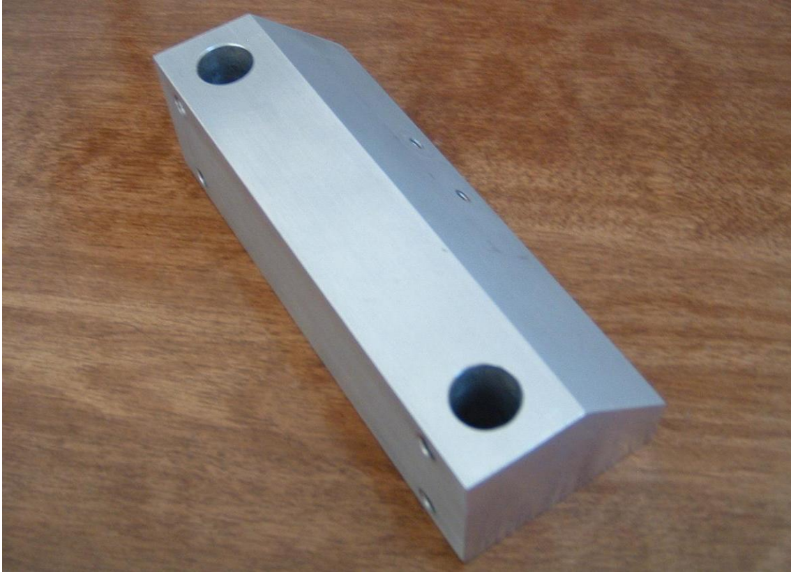
Figure 3-7: Picture of angle mount for beam steering mirror
