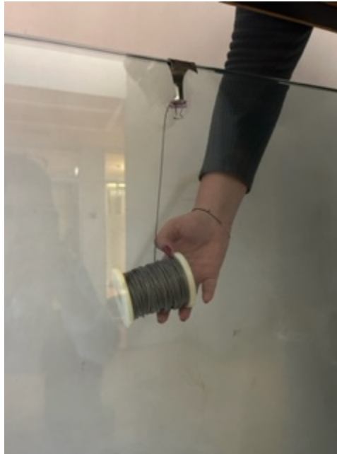
Figure 21: S hook testing on stair glass and aluminum wire
