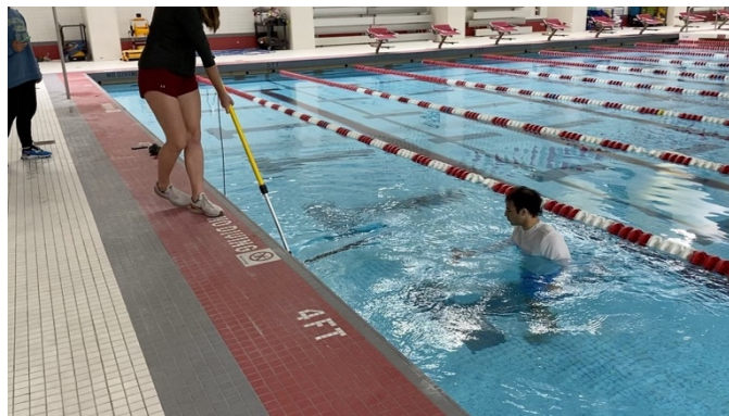
Figure 61: Image of pool testing where we moved the whole system through the water by walking along the pool deck
