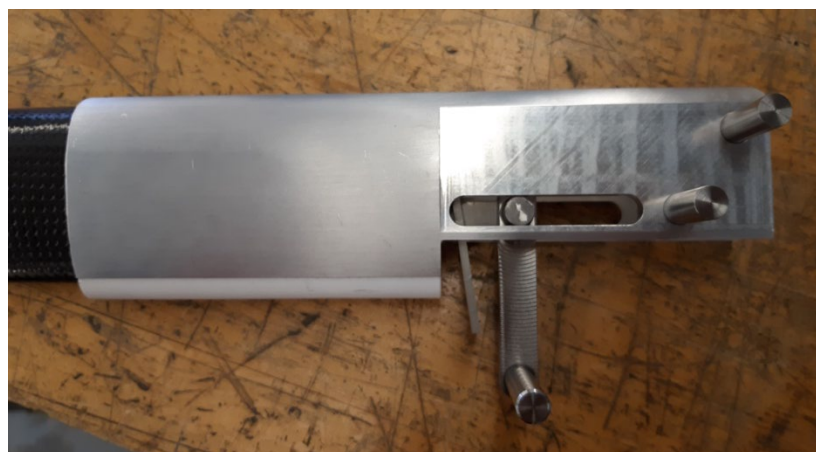
Figure 39: Manufactured clamp opener with offset arm
