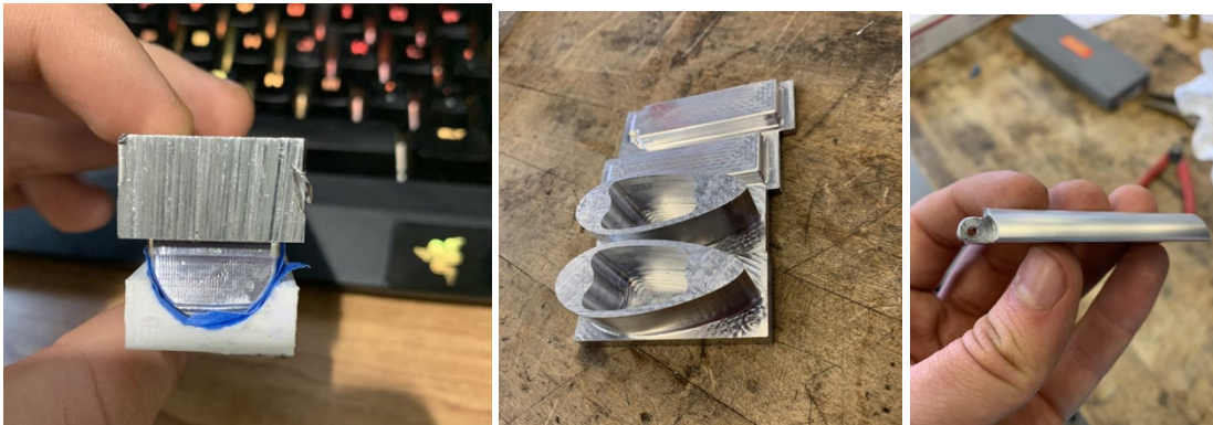
Figure 45: Initial trigger operation one (left), actual first trigger operation (middle), final trigger piece (right)
