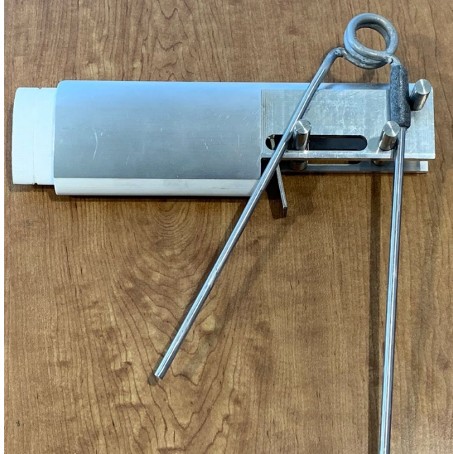
Figure 41: Final clamp opener version after testing
