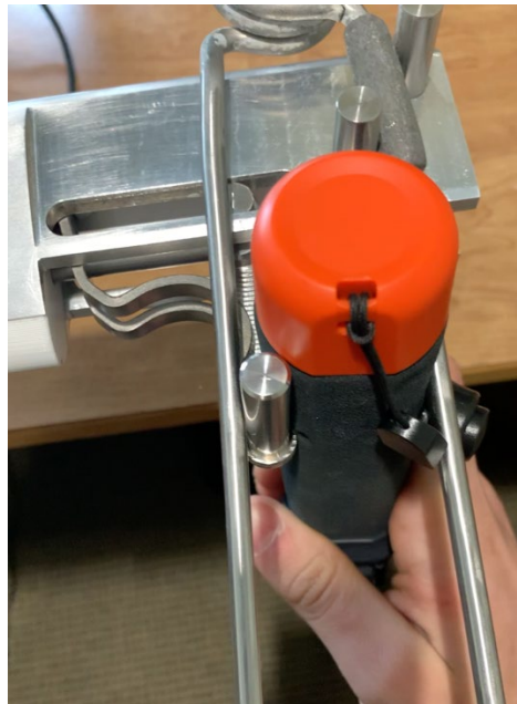
Figure 40: Offset arm wedged against object, preventing clamp from closing completely
