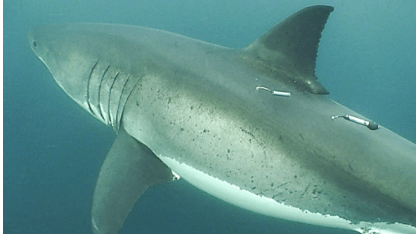
Figure 9: Acoustic tag on great white shark in the front with PSAT in the back [28]
