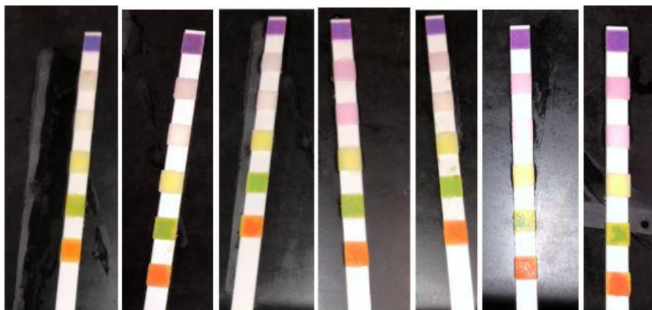
Figure 16. Water quality test strips (from left to right: Influent, Aerobic, Anoxic, Anaerobic Primary Effluent, Final Settling, Final Effluent)
