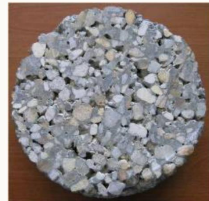
A close-up of permeable concrete.
