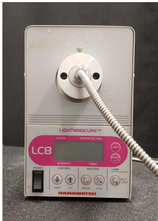
Figure 38. The UV light source used in the experiment 9 (LightningCure LC8).
