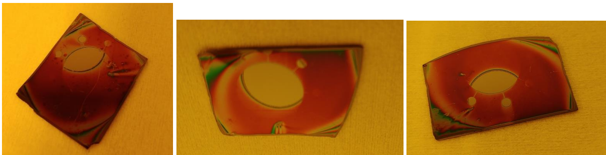
Figure 42. Samples after developing with 0.26 N TMAH developers.
