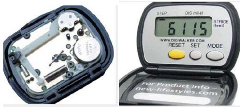
Figure 3: Digiwalker Pedometer boasts accurate counting due to state of the art lever arm sensor, a tightly coiled spring for increased accuracy, and special features to reduce noise and corrosion [18].
