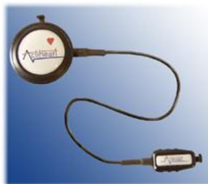
Figure 9: Actiheart monitor which uses heart rate and accelerometry to output energy expenditure. The device slips onto two chest electrodes and has a triaxial piezoelectric accelerometer [24].
