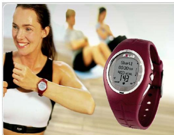
Figure 5: Polar heart rate monitor with chest strap and wrist device. Consists of a transmitter belt worn around the chest and a device that is attached to the wrist which displays energy expenditure parameter output [18].
