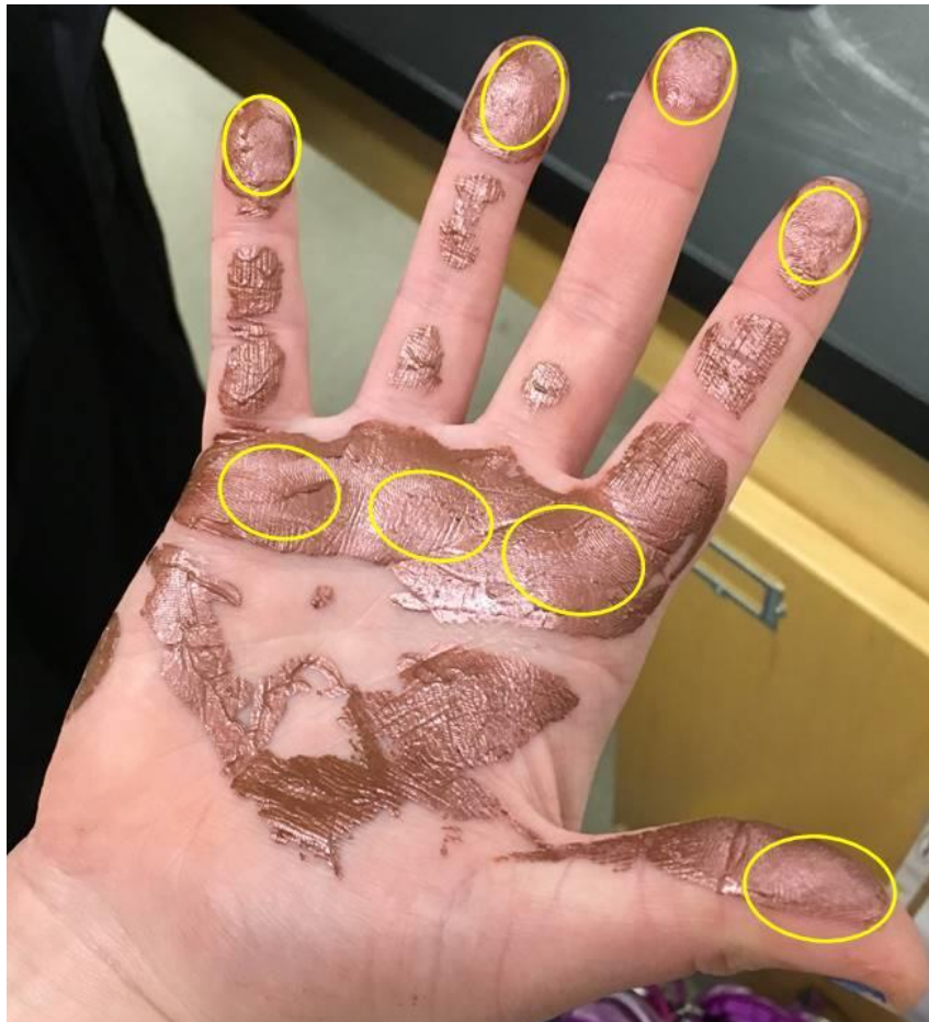
Figure 35: Based on the location of the paint on the hand after typing on a opening a lever door handle, the sensor locations for the hand were determined as follows: 4 sensors on each of the 4 finger pads, 1 sensor on the pad of the thumb pad, and 3 sensors at the top of the hand, below the fingers. The determined sensor locations can be seen in the yellow indicators on the hand.
