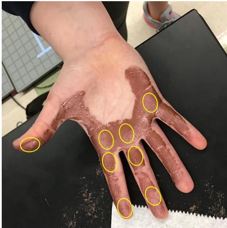
Figure 32: This figure shows the paint as a result of opening a jar with non-dominant hand holding the side of the jar. Based on the location of the paint on the hand after opening a jar, the sensor locations for the hand were determined as follows: 1 sensor on the pad of the thumb, 1 sensor on the pad of the index finger, 1 sensor on the middle phalanx of the middle finger, 2 sensors on the proximal phalanx of the index and middle fingers, and 3 sensors across the top of the palm. The determined sensor locations can be seen in the yellow indicators on the hand.
