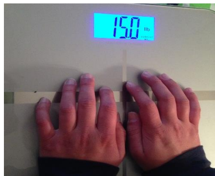
Figure 22: Tying force testing using bathroom scale.
