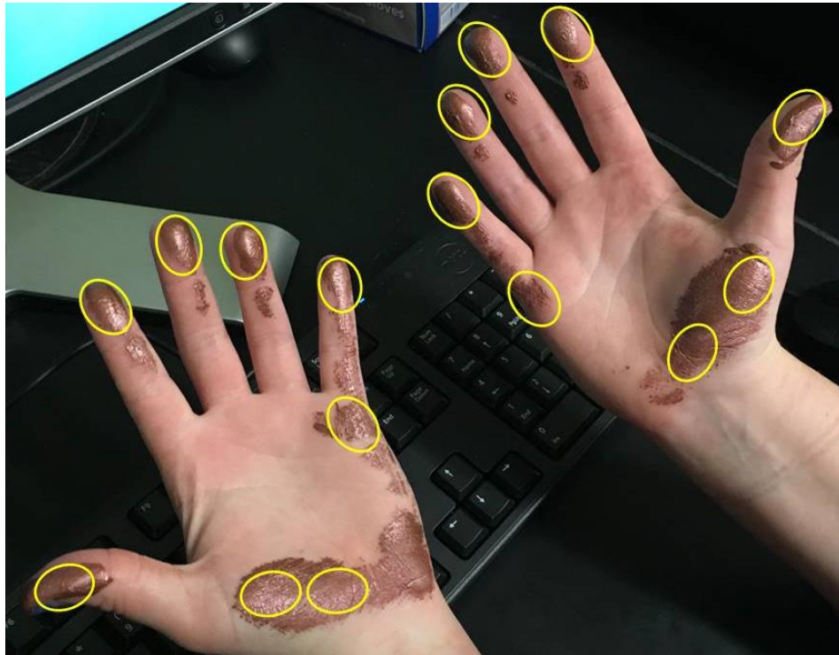
Figure 34: Based on the location of the paint on the hand after typing on a keyboard, the sensor locations for the hand were determined as follows: 4 sensors on each of the 4 finger pads, 1 sensor on the side of the thumb pad, 2 sensors at the bottom of the hand, above the wrist, and 1 sensor on the side of the hand below the small finger. The determined sensor locations can be seen in the yellow indicators on the hand.
