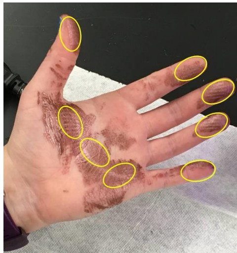
Figure 31: This figure shows the paint as a result of opening a jar with the dominant hand on top of the jar lid. Based on the location of the paint on the hand after opening a jar, the sensor locations for the hand were determined as follows: 4 sensors on each of the 4 finger pads, 1 sensor on the side of the thumb pad, and 3 sensors across the palm of the hand. The determined sensor locations can be seen in the yellow indicators on the hand.
