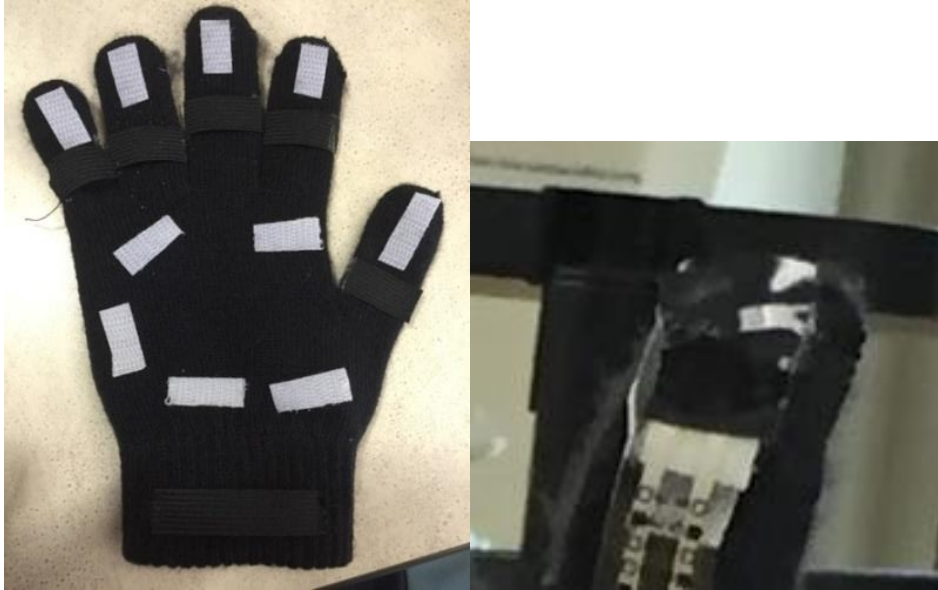
Figure 53(left): The glove with Velcro® and elastic loops to hold the sensors. To see a bill of materials and instructions on how to make this glove see Appendix D.
