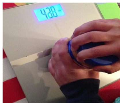
Figure 23: Jar opening force testing using bathroom scale.
