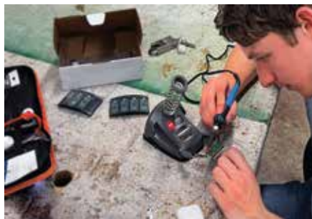
Figure 19: Banksia IQP student soldering heat sensors for their deliverable
