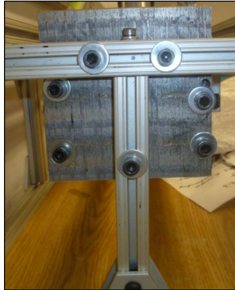
Figure 32: Rear dropout base plate fixtured to test rig frame.
