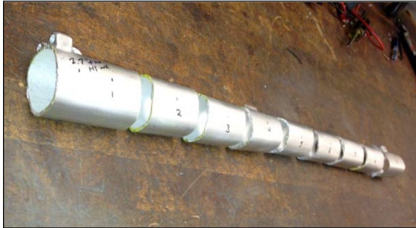
Figure 19: Sectioned top tube for cross section measurements.
