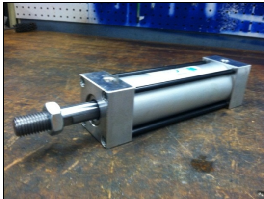
Figure 31: Air cylinder used to exert forces onto tested bike frame.
