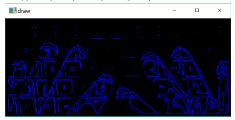
(b) The Canny algorithm detects edges in the segmented imageFigure 3.5: The steps in the "FindHands" function
