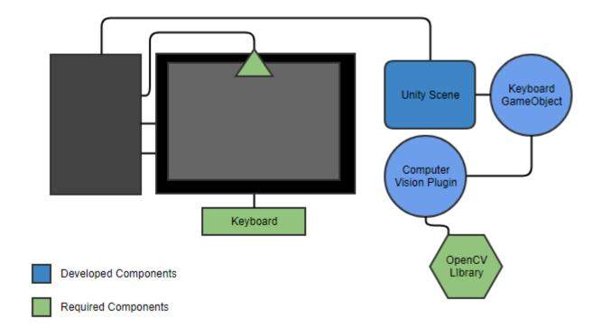
**Figure 3.1:** A diagram illustrates the components of the system implemented and how they fit together.
