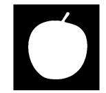
**(b)** *A mask created by thresholding the image for the color green.*
