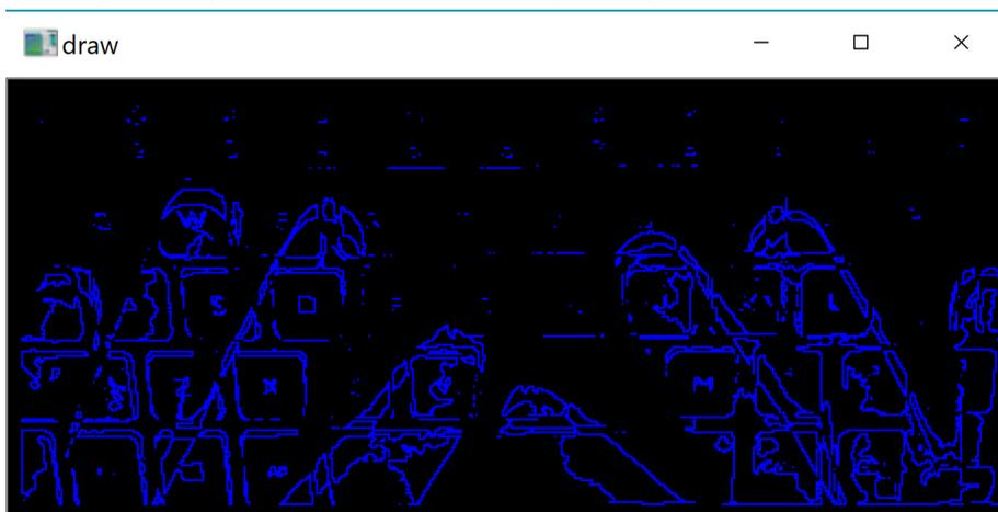
(b) The Canny algorithm detects edges in the segmented image
