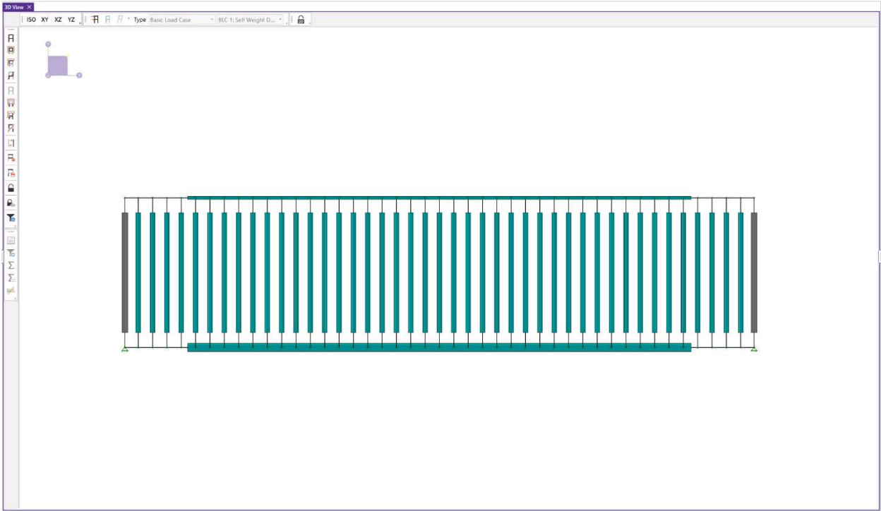
Model 2: Structural Truss with Verticals of a 40-foot High-cube Shipping Container with Member Renders
