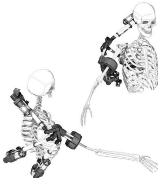
FIGURE 2.8: Theoretical image of the parallel actuation and passive slip interference device [24]
