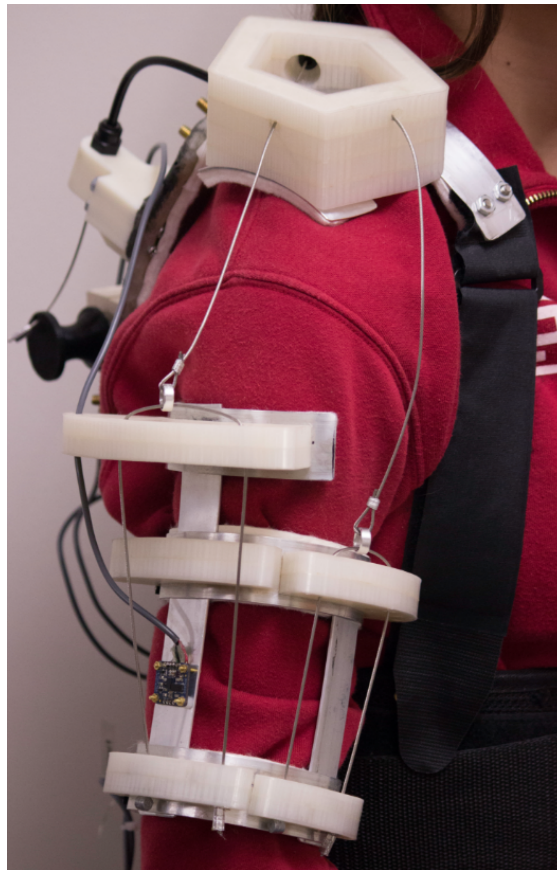
FIGURE 6.6: Pulley Cable System
