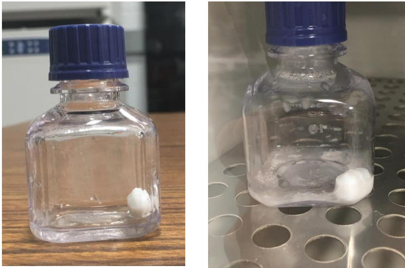
Figure 20. Left panel: NIPAAm dissolves in cold PBS. Right panel: Clumping of NIPAAm solution after 20 minute at 47°C
