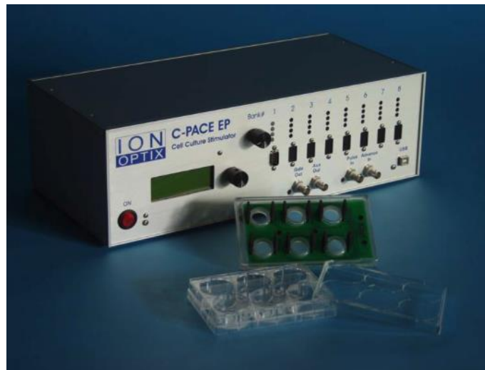
Figure 16: IonOptix C-Pace EP programmable multi-channel power source and 6-well electrode plate lid [38]
