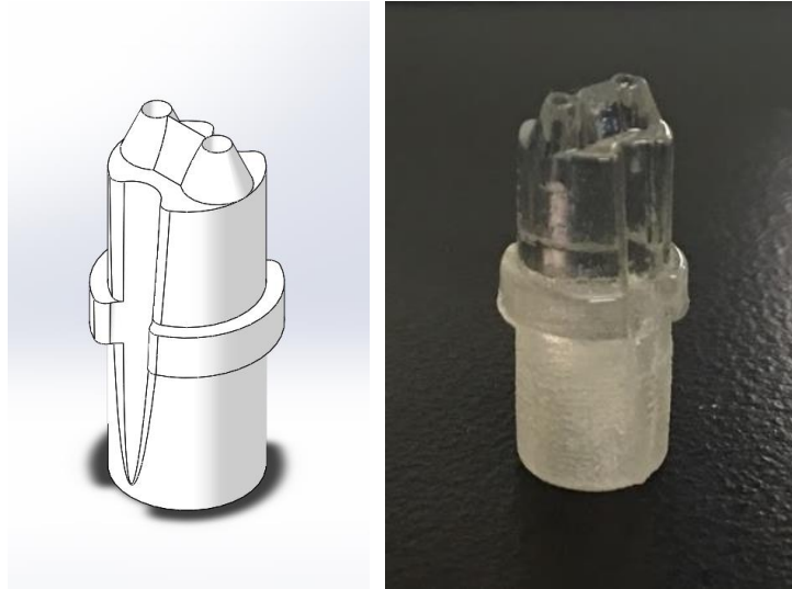
Figure 21. Left panel: CAD model of V-shaped NIPAAm mold. Right panel: image of 3D printed mold.
