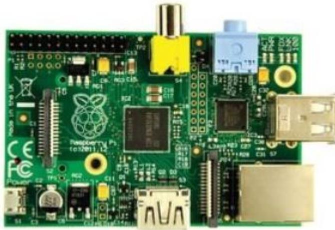
Figure 14: Raspberry Pi B Model
