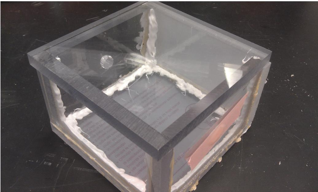
Figure 12: Polycarbonate Enclosure Box
