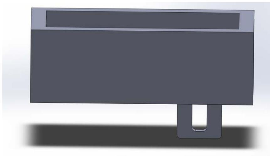
Figure 8: Side view of electromagnet dish
