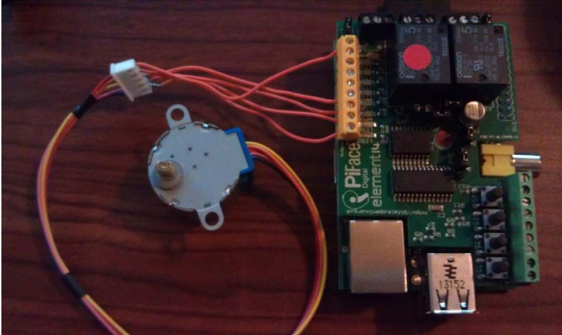
**Figure 17: Full Construct of Mechanical Actuation Controller and Stepper Motor**
