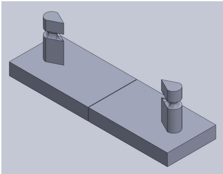
**Figure 6: Inner mold with tear drop posts**
