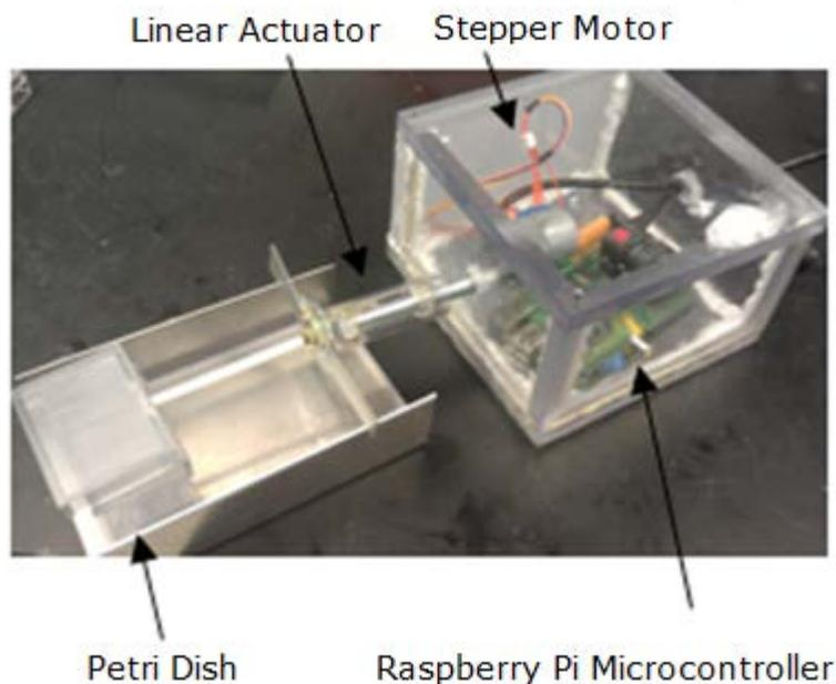
**Figure 13: Final Design Components**
