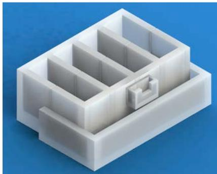
**Figure 11: 2-Piece pool system with slot for attachment to mechanical actuator**
