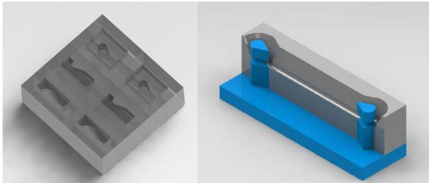
Left: Veroclear negative mold. Right: Representation of post and seeding channel system. Blue: PDMS post and Grey: agarose channel
