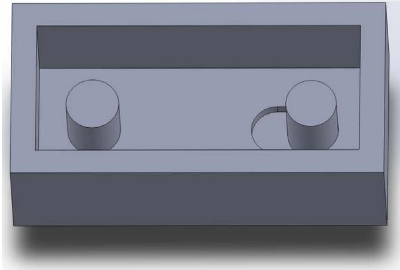
Figure 7: Top view of electromagnet dish
