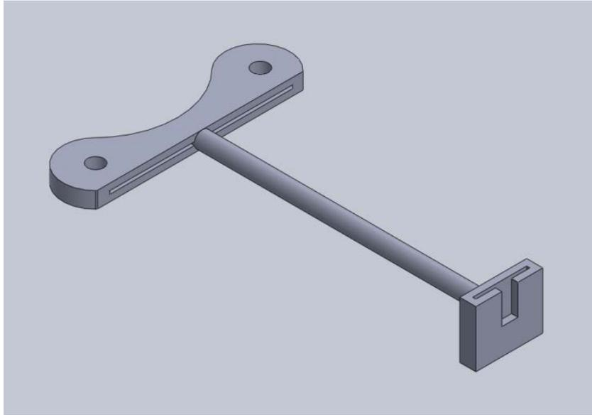
**Figure 9: Push arm for connection with syringe pump**
