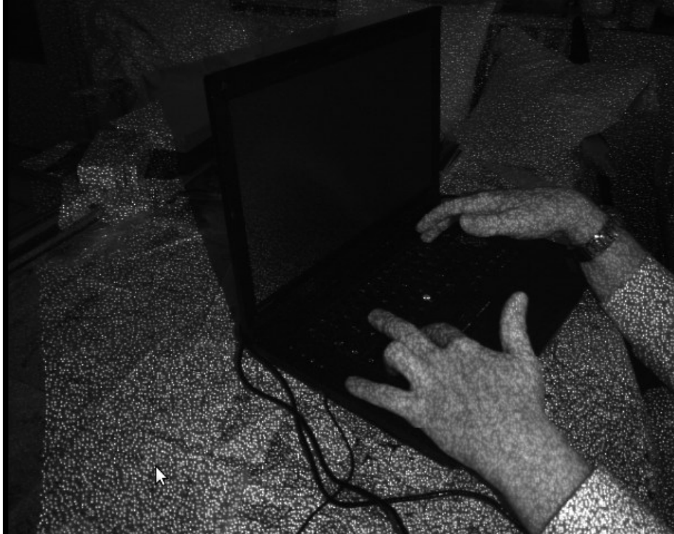
Figure 7: Microsoft Kinect IR Projection [6]
