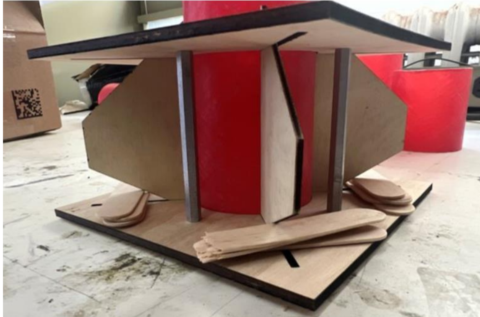
Figure 26 New Fin Jig in Use with New Fins
